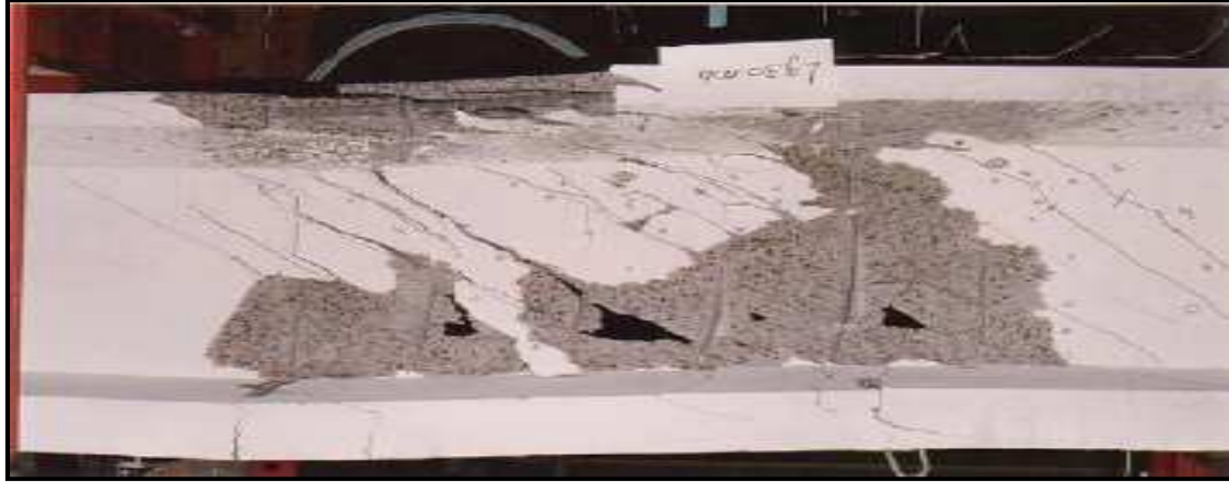
Figure 5.3. Sudden web compression failure due to large amounts of shear reinforcement (Joint Research Centre, 2008)
