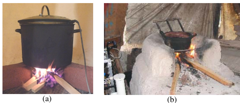
Figure 4. Traditional cooking methods: (a) three-stone fire, (b) traditional cookstove (Reprinted with permission from Roden, C. A., Tami C. Bond, Stuart Conway, and Anibal Benjamin Osorto Pinel. 2006. “Emission Factors and Real-Time Optical Properties of Particles Emitted from Traditional Wood Burning Cookstoves.” Environmental Science & Technology 40 (21) (November 1): 6750–6757. © 2006 American Chemical Society.).
