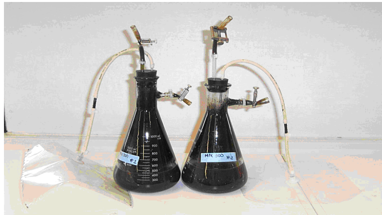
Figure 3.6 Configuration of semi-continuous anaerobic digesters
