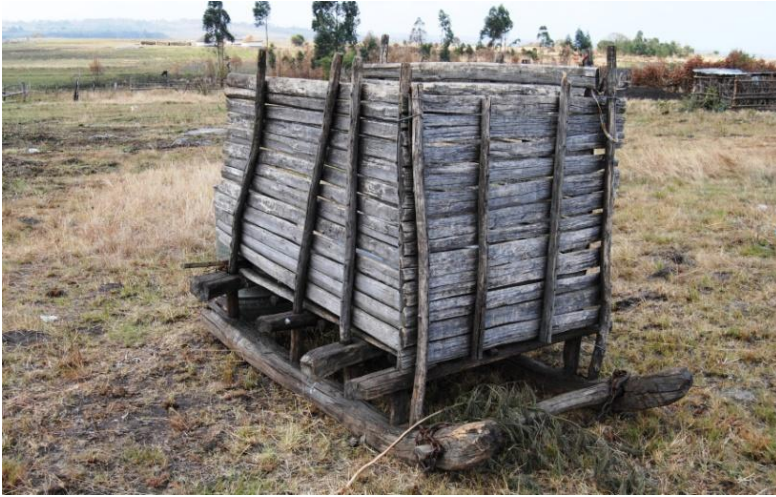
Figure 33. Slatted sled for hauling building materials such as clay bricks. Sigidi
