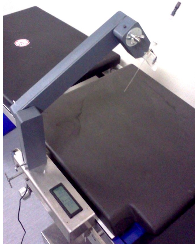
Figure 4.16: Photograph of the assembled needle-positioning device attached to a typical operating theatre bed
