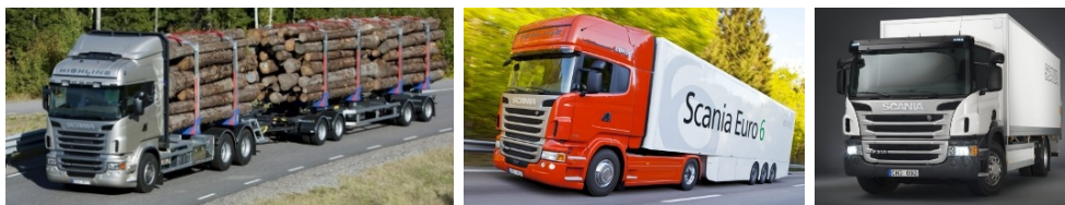
Figure 1.2: Three different but commonly used vehicle configurations: a long-haulage timber truck and trailer, a streamlined tractor-semitrailer combination and a smaller distribution truck. Images courtesy of Scania CV AB.
