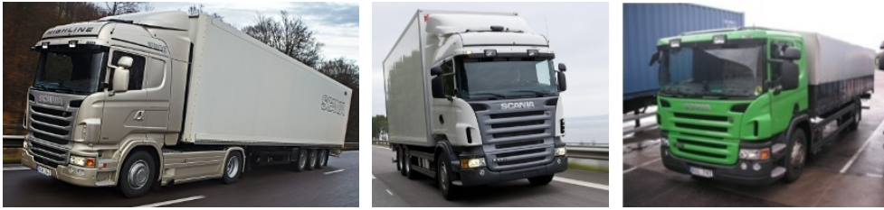
Figure 5.1: The three vehicle configurations that was used in the experiments. A tractor-semitrailer combination (test vehicle A), a box-body truck (test vehicle B) and a smaller distribution truck (test vehicle C). Images courtesy of Scania CV AB.
