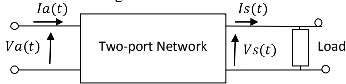
Figure 7.20 : Two-port network for rectangular unimorph beam
