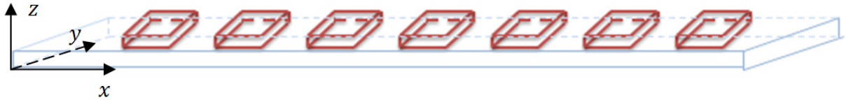
Figure 3. 4: non-collocated piezoelectric patches bonded on a beam of the same width
