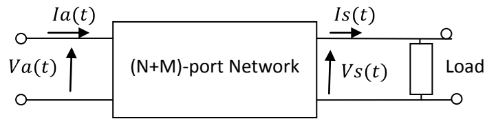
Figure 7.21: (N+M) port-network for thin plates with non-collocated piezoelectric patches actuators/sensors
