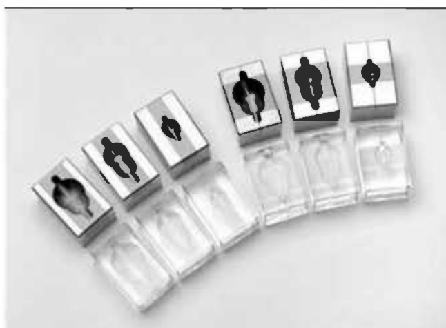
Figure 3.5 The brain matrix for coronal brain slices preparation spaced 1 mm apart. The brain was placed on the matrix and sliced by blades by cutting at every 2-mm intervals. Photo adopted from manufacturer website.
