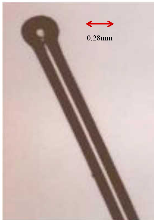
Figure 3.1 The poly-L-lysine coated intraluminal filament head ( 0.38 \pm 0.02\text{mm} ) with cylinder diameter of 0.28 mm as seen under microscope (40X magnification).
