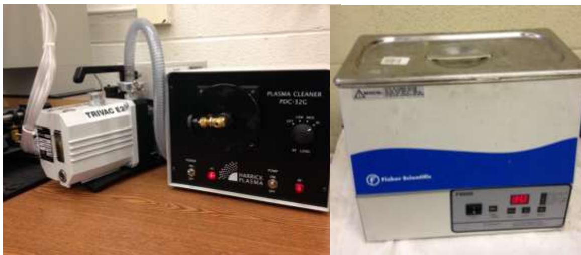
Figure 3.3 – a) Harrick Plasma Cleaner PDC-32G and b) Fisher Scientific FS60D Sonicator used in experiments.
