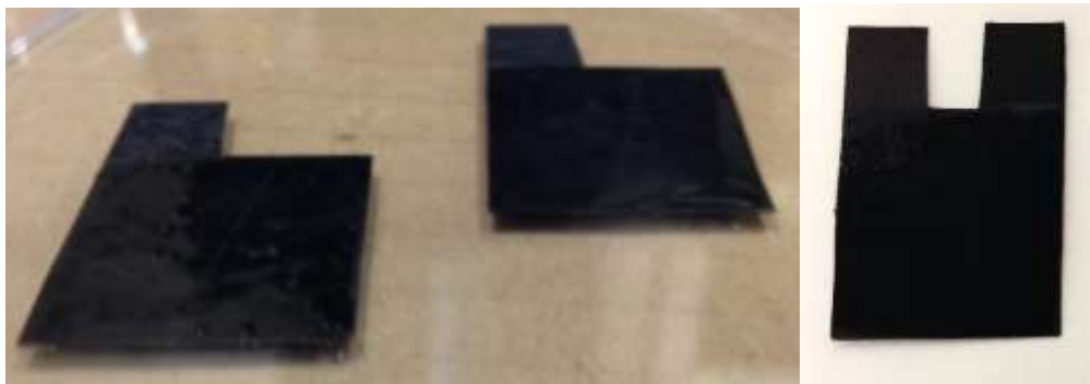
Figure 3.7 – Supercapacitor electrodes while they were drying, and the finished product.
