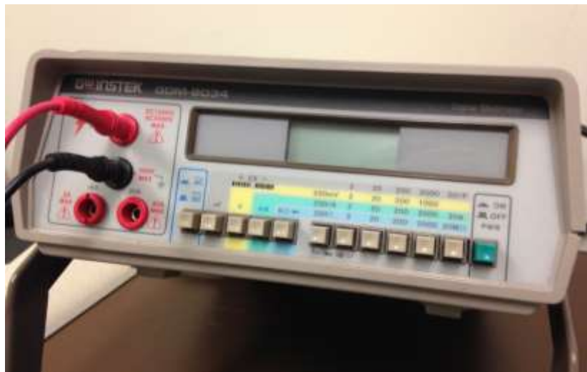
Figure 3.11 - GWINSTEK GDM-8034 Digital Multimeter used in the resistance measurements.
