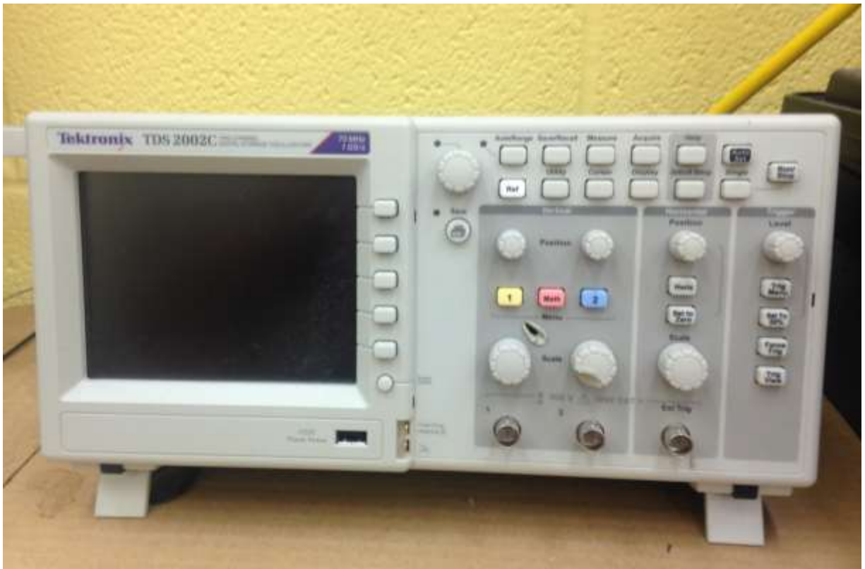
Figure 3.12 - Tektronix TDS 2002C Oscilloscope used in observing charge and discharge.
