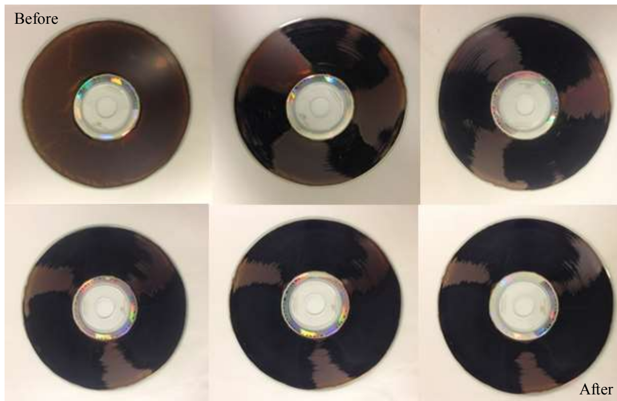
Figure 3.5 – The burning steps of graphene oxide nanofilm.
