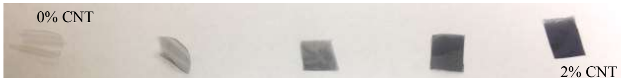
Figure 3.6 – Photographs showing the electrolyte thin films.
