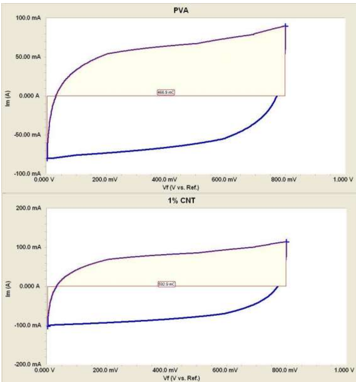
Figure 4.4 – Calculating the charge accumulated in (a) PVA/ H_3PO_4 and (b) PVA/1%CNT/ H_3PO_4 .
