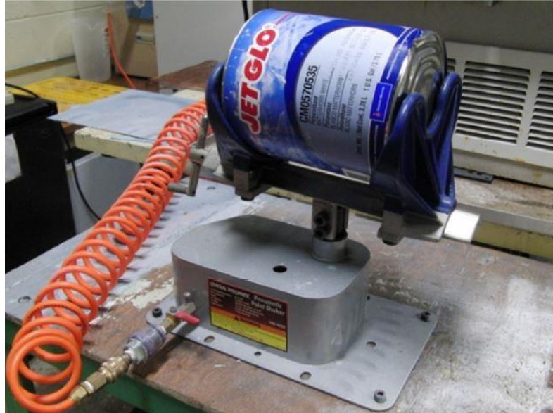
Figure 8: Pneumatic Paint Shaker Used to Mix Primer and Top Coat Before Paint Application.
