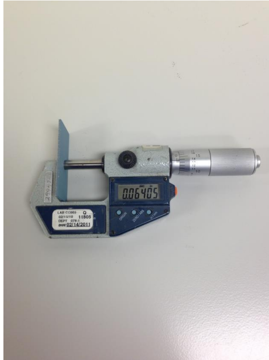
Figure 32: Measurement of Coating Thickness Using the Mitutoyo 293-725 Digimatic Micrometer.
