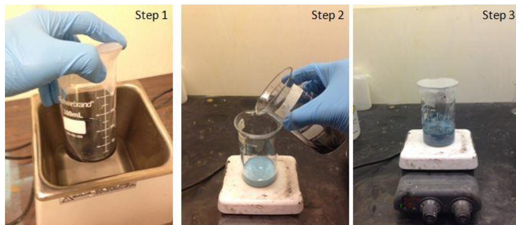
Figure 29: Preparation of Base Coat Containing Various Percentages of Nanoadditives. Step 1) Mix epoxy adduct with primer by high power sonification for 30 minutes Step 2) Mix the epoxy primer with the epoxy adduct Step 3) Blend the mixture on a hot plate for 4 hours at room temperature
