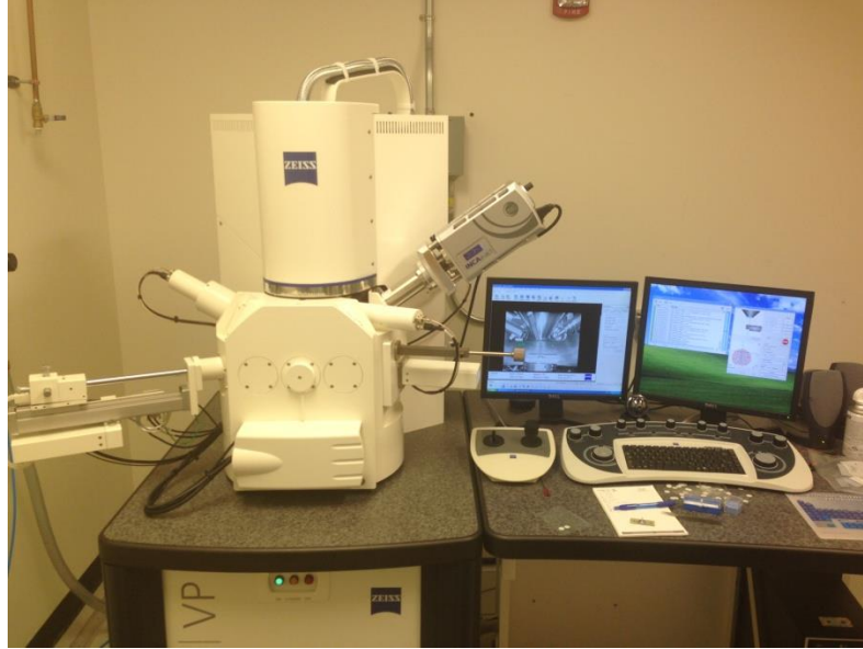
Figure 20: SIGMA Series of Field Emission Scanning Electron Microscope Used to Image the Surface of Nanocomposite Coatings Containing Silanized and Non-silanized Graphene Particles.
