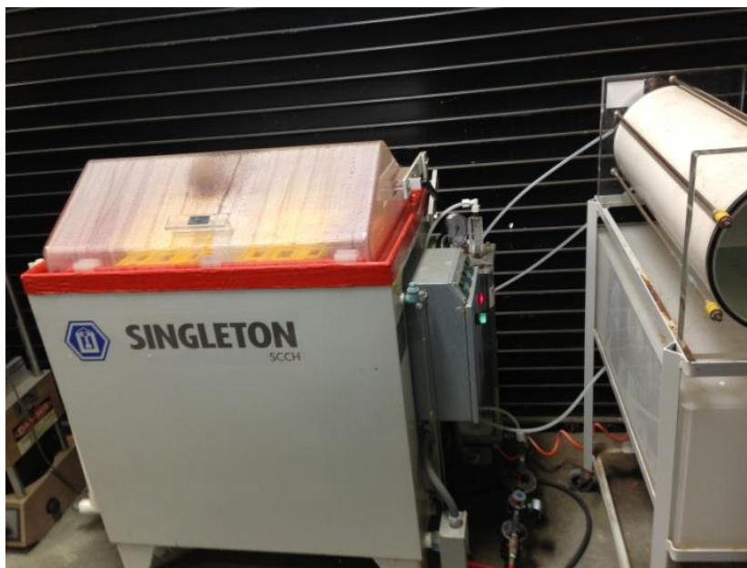
Figure 16: Salt Spray Chamber Used to Simulate the Corrosive Environment for Nanocomposite Coatings.
