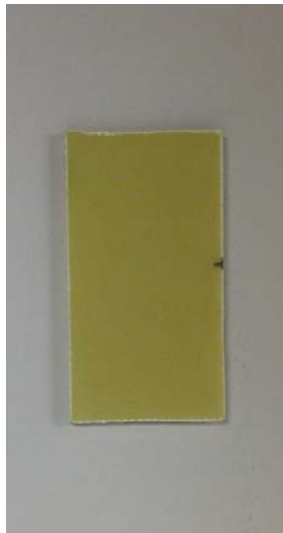
Figure 5: One 1"x2" GFRC Test Coupon Obtained from NIAR Composite Lab.
