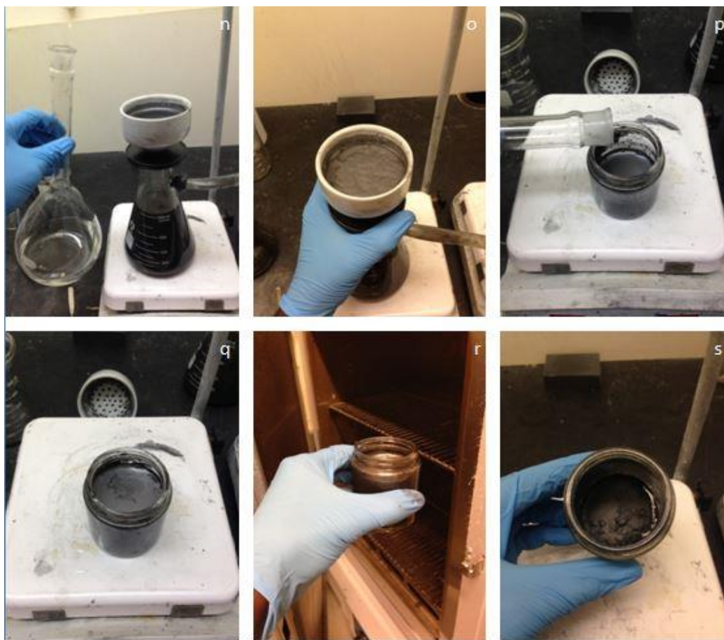
Figure 24: Silanized Graphene Preparation (Part 3); n) Rinse the graphene with 500 ml DI water o) Let all the water seep through the filter p-q) Collect the graphene in a small container and add more DI water r) place the container in the oven at 70 °C overnight s) Collect the silanized graphene
