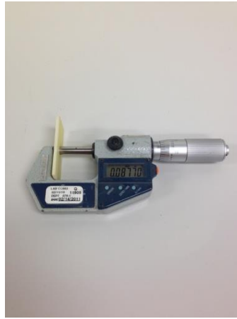
Figure 14: Mitutoyo 293-725 Digimatic Micrometer Used to Control the Coating Thickness.
