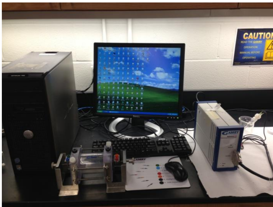
Figure 17: Gamry Reference 600 Potentiostat Used to Evaluate the Nanocomposite Coatings.
