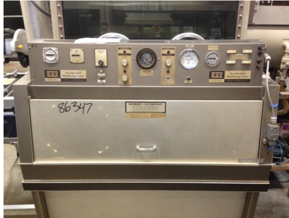
Figure 15: QUV Accelerated Weathering Cabinet Used to Simulate the Weathering of Nanocomposite Coatings.
