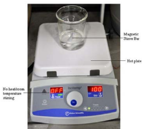
Figure 12: Hot Plate from Fisher Scientific Used to Mix the Coating System.
