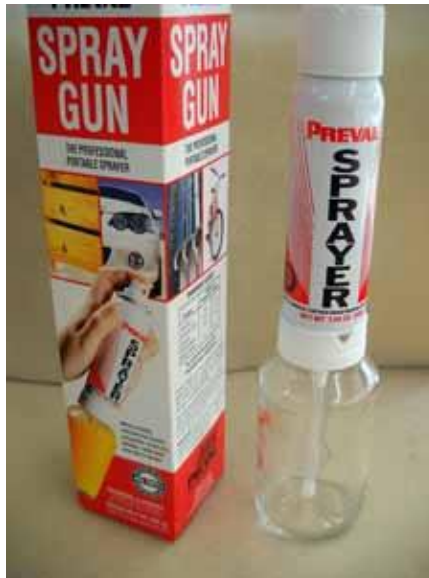
Figure 9: Preval Spray System Used to Spray Paint Test Samples.
