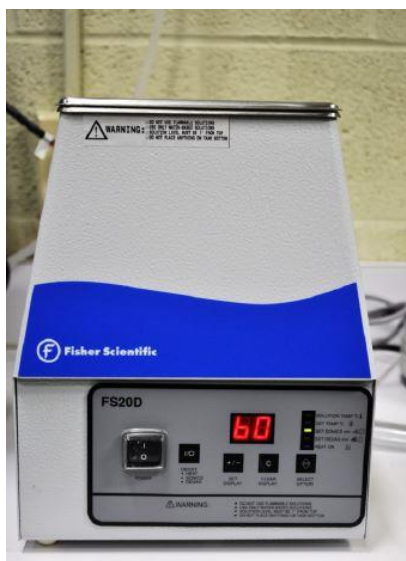
Figure 13: Fisher Scientific FS 200 Sonicator Used to Mix the Nanoparticles Inside the Coating System.
