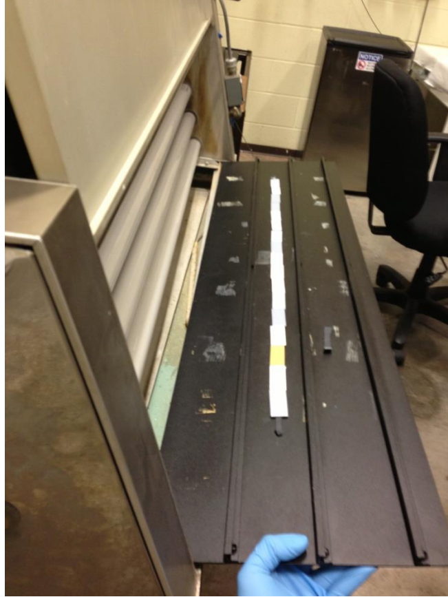
Figure 33: UV Degradation Test Using the QUV Weathering Tester.
