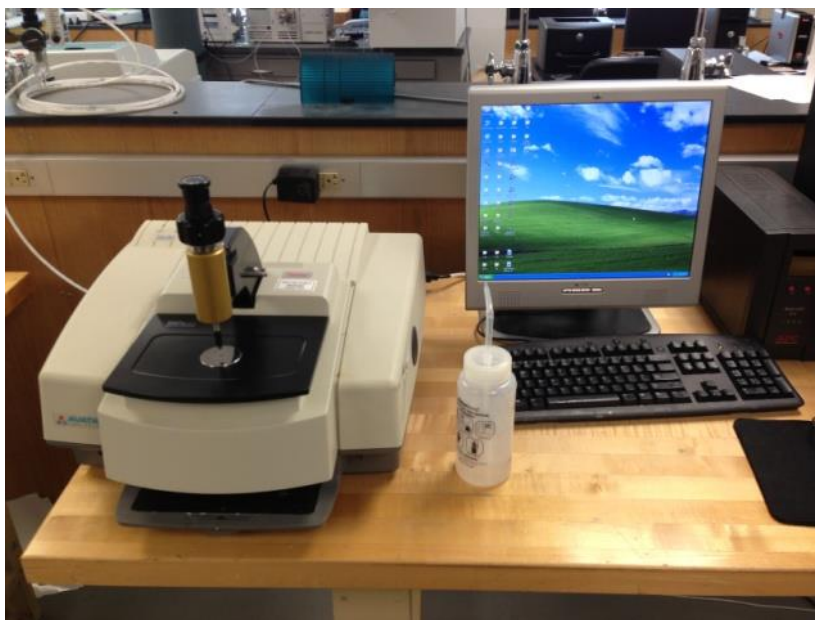
Figure 18: Thermal Nicolet Magna 850 IR Spectrometer Used to Perform FTIR Studies.
