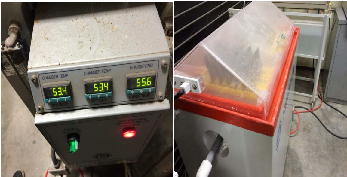
Figure 25: Test Samples Undergoing Humidity Exposure in Moisture Chamber
