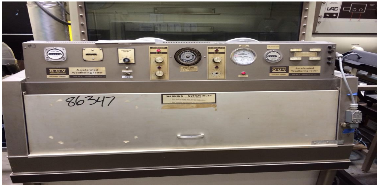
Figure 22: UV Chamber Setup
