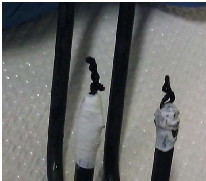
Figure 4.22: 100 Yarn CNT attached to probe
