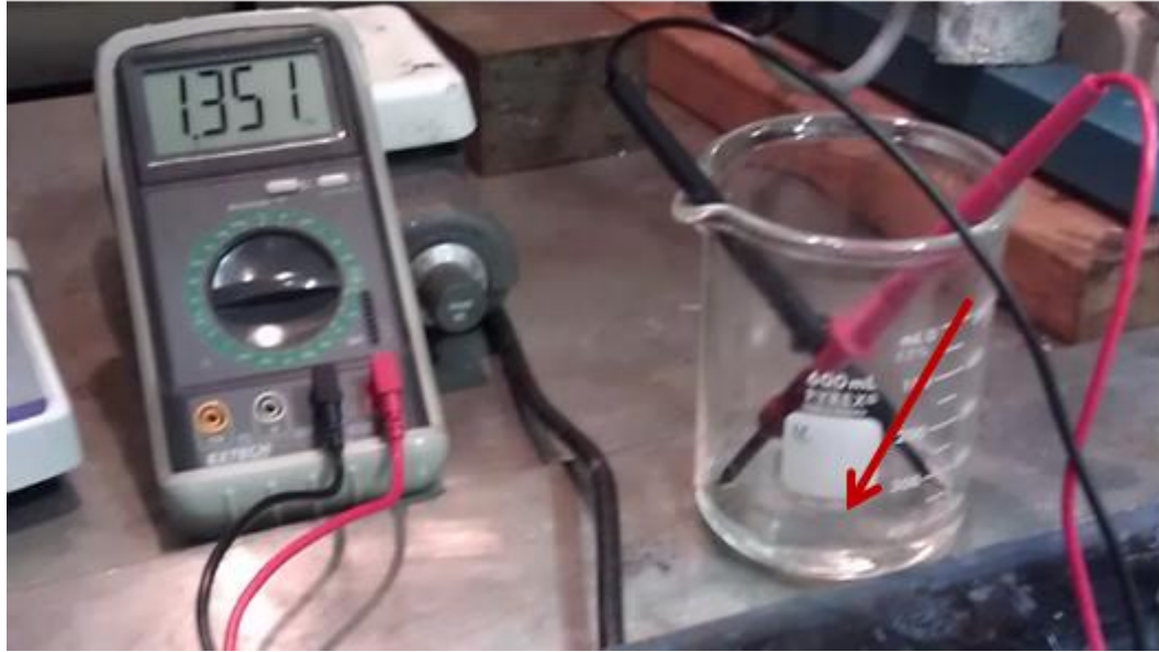
Figure 3.3: Typical emersion of CNT wire in acid bath.
