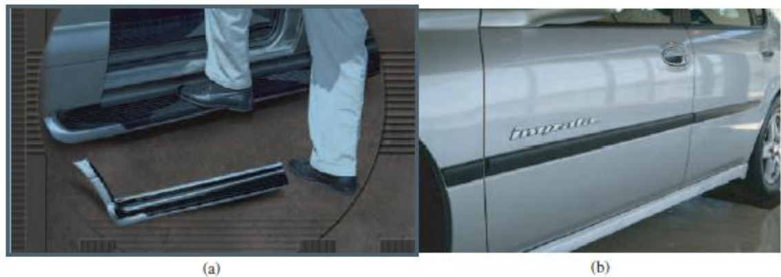
Figure 1.3: TPO Nanocomposite: Application for automotive parts: a) 1st commercial lunch b) 2 nd nanocomposite application on Chevy Impala [3].
