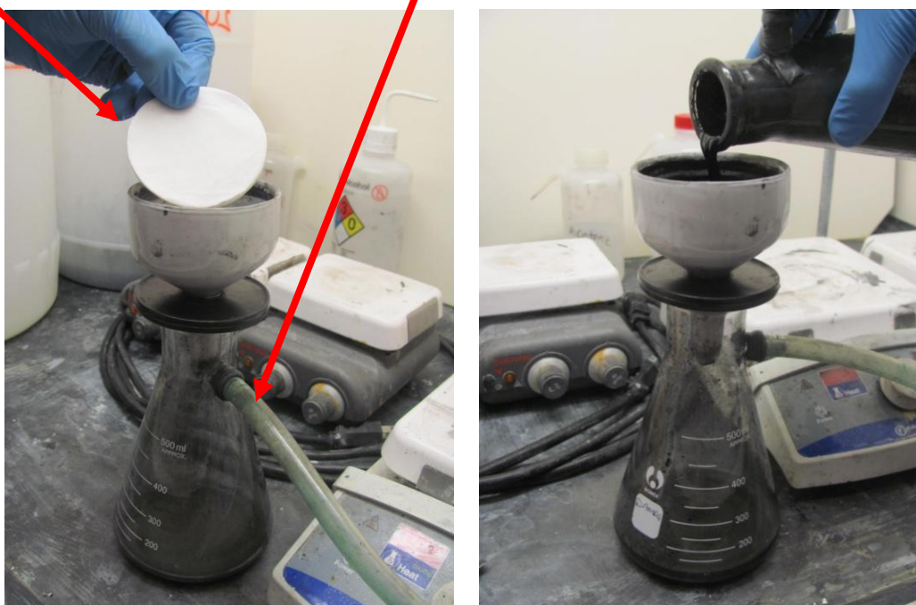
Figure 3.26 a: Placing the Buchner funnel on the Buchner flask and turning on the vacuum, placing a filter into the funnel and pouring the solution into the funnel
