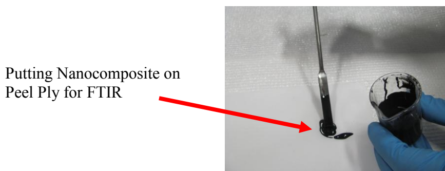
Figure 3.34: From left to right process of making specimen for FTIR on a piece of Peel ply
