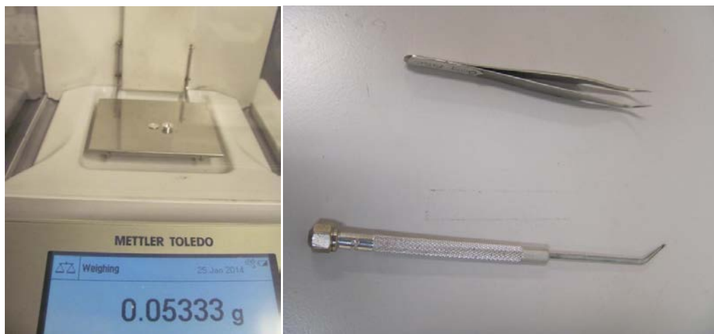
Figure 3.18: High Accuracy Weight Scale (left) Dental Probe Tool (right and bottom) and Laboratory Tweezer (right and top)
