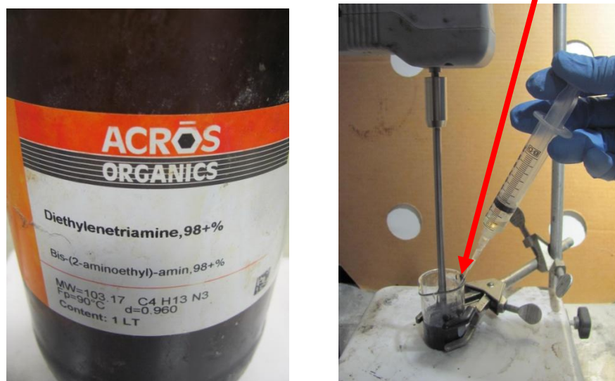
Figure 3.30: Adding Diethylenetriamine,98+% (DETA) curing agent to the carbon black nanocomposite and making it ready for testing
