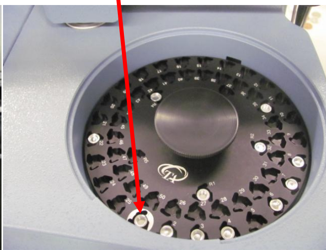
Placing the Pan on DSC circular rack
