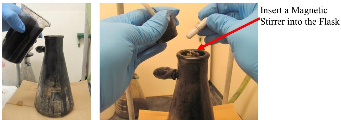
Figure 3.25 a: Pouring the mixture in to flask (left) and Inserting a magnetic stirrer into the flask (right)
