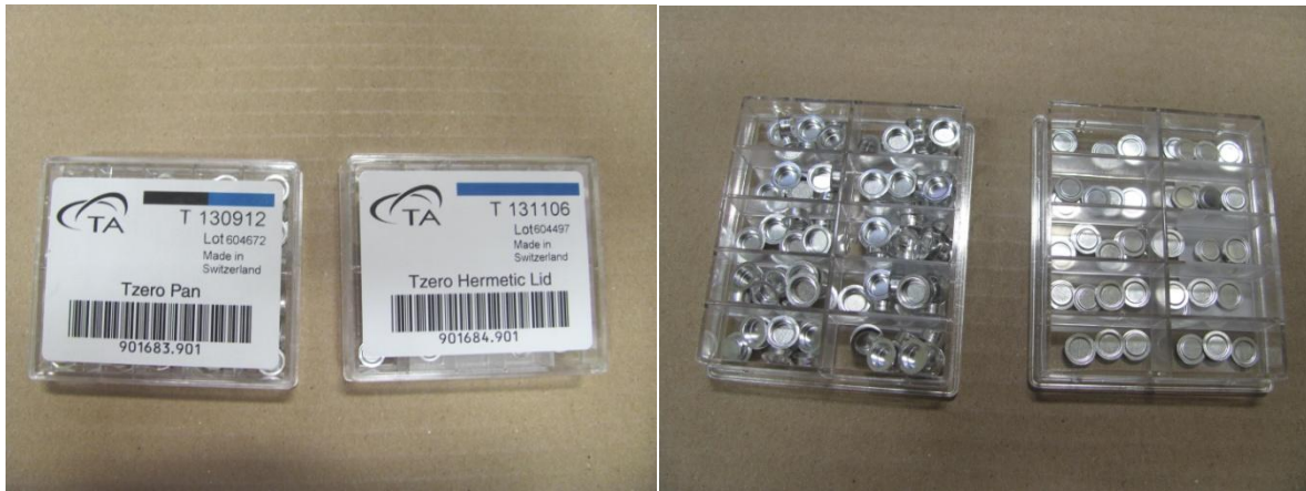
Figure 3.17: Tzero Pan (left side of each picture) and Tzero Hermetic Lid (right side of each picture)
