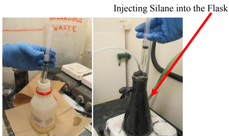
Figure 3.25 b: Drawing silane with a syringe (left) and injecting into the flask through a prepared hole on the cap (right)
