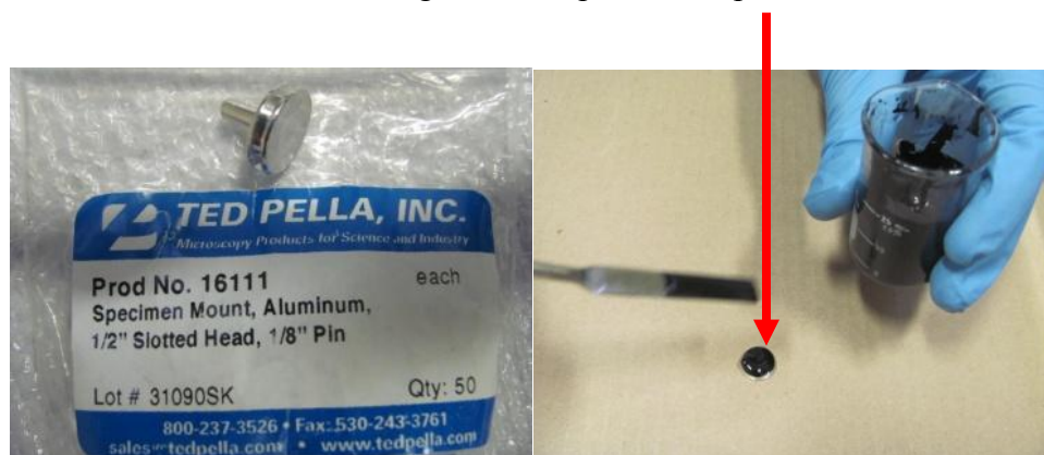
Figure 3.31: Aluminum Specimen Mount 1/2" Slotted Head, 1/8" Pin (left) Putting Nanocomposite on the Mount for SEM
