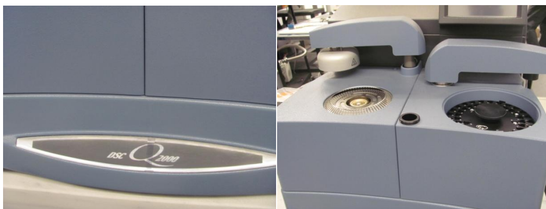
Figure 3.20: DSC Q2000 was used to measure the degree of cure (DOC)
