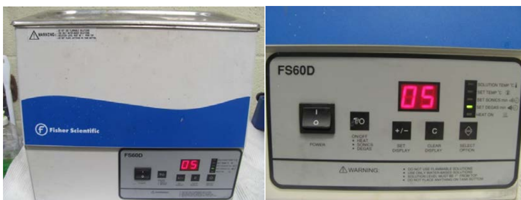
Figure 3.5: Ultrasonicator bath was used for even dispersion of carbon black in ethyl alcohol
