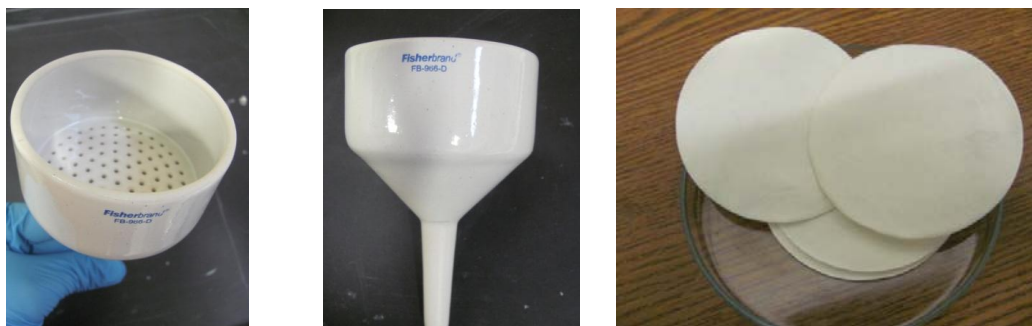
Figure 3.10: Buchner Funnel (left and middle) and Filter Paper (right) used for Filtration
