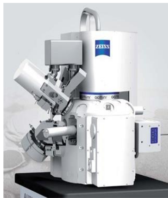
FIGURE .4.10 SEM apparatus
