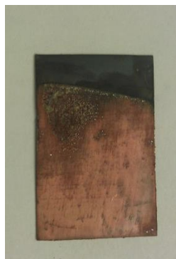
FIGURE 5.17 Powdery coating at low conductivity
