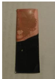
FIGURE 5.11 Coating at 3.75E2 \text{ A/m}^2 for 30 minutes at 4.23 \text{ S/m}^2
