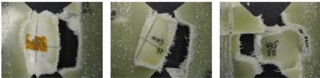
Figure 10. Complex failure modes across the sections of the coupon Newport SWGF at different stroke rates [5]
