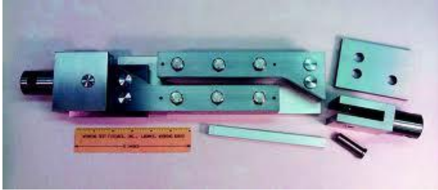
Figure 7. Two-rail shear test fixture [12]
