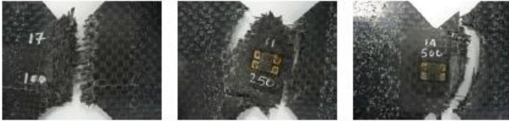
Figure 9. Complex failure modes across the sections of the coupon Newport PWCF at different stroke rates [5]
