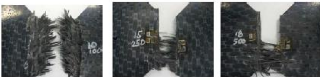
Figure 8. Failure modes across the minimum section of the coupon Cytac PWC/T300/3KNT at different stroke rates [5]
