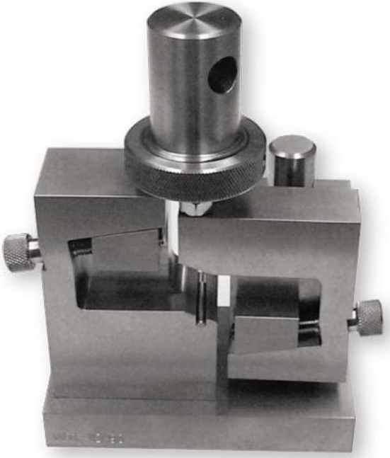
Figure 6. Iosipescu shear test fixture [12]
