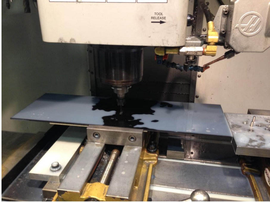
Figure 3-8 Test article in flaw machining process
