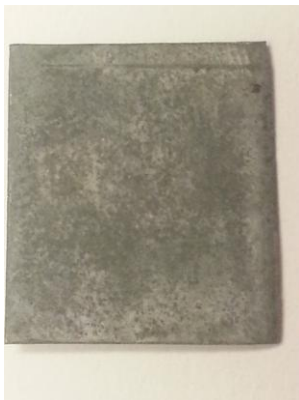
Fig. 4.2 Camera image of zinc immersion coated AZ31 magnesium alloy
