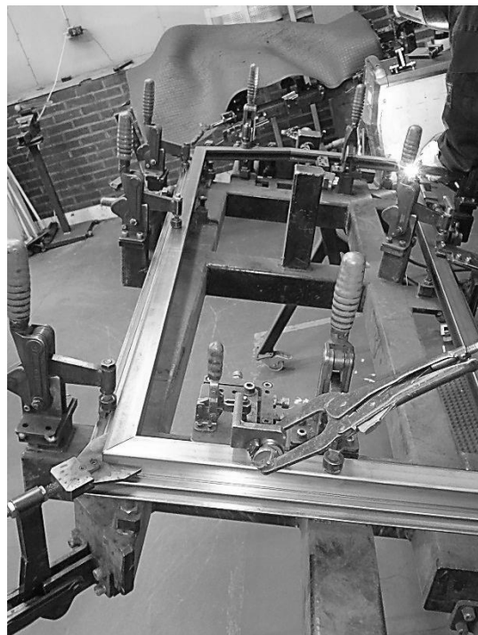
Figure 8: Steel profiles in fixture for door frame.
