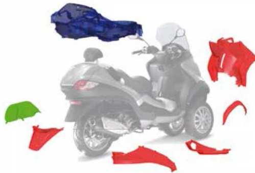
Figure 4.2, Recycled pigmented polypropylene parts of a Piaggio scooter [12].
