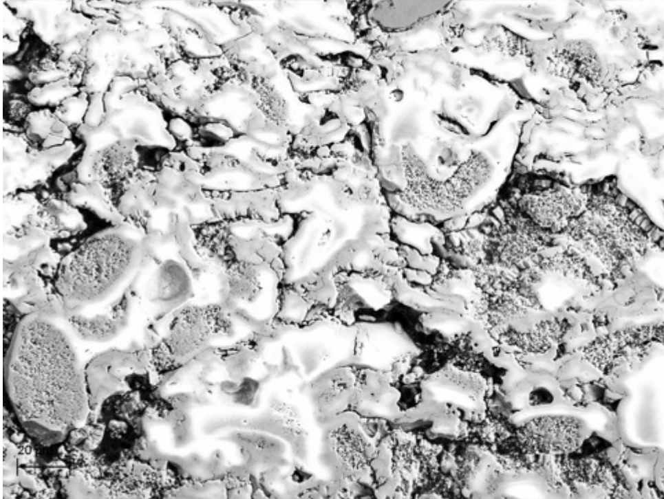
Figure 46 nano 8YSZ coated onto d5s showing the coatings nanozones and micro cracked matrix.
