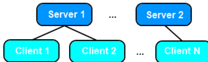
Figure 17. The multiple server architecture.
