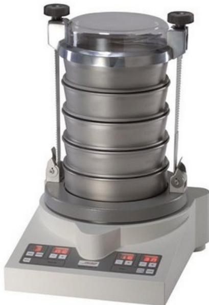
**Figure 16.** The mechanical shaker involving a nested column of sieves. (Fritsch 2013)
