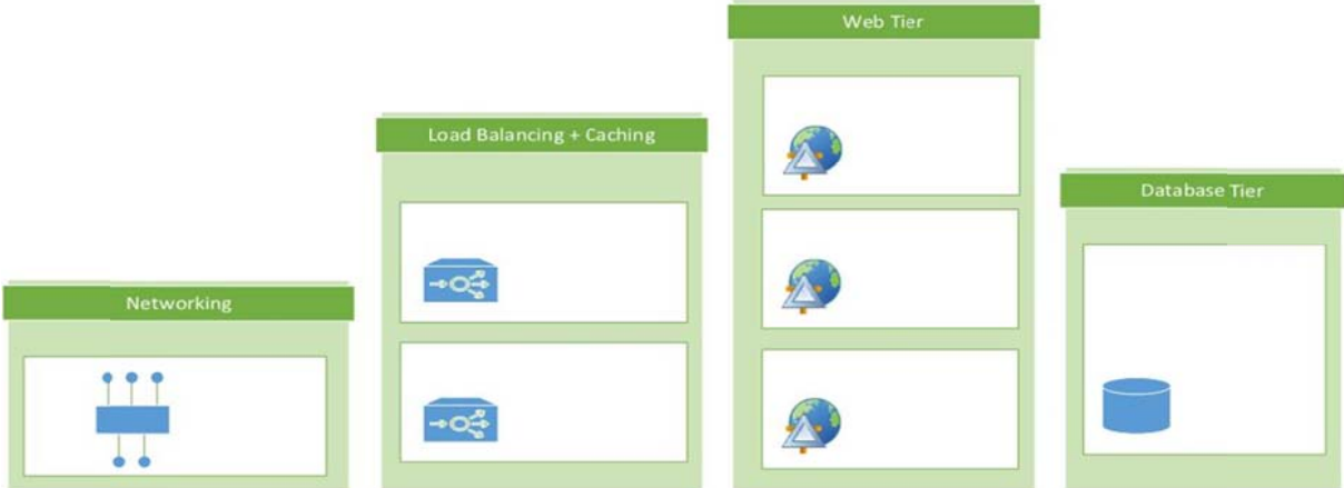
Figure 2-2: Horizontally scaled load balancing and web-tier and vertically scaled database tier (Adapted from Figure 2, page 9 of [21])
