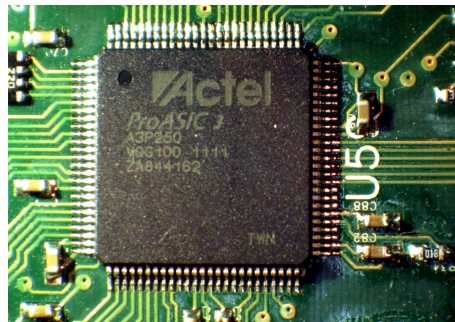
Figure 7: Actel A3P250 FPGA used for image processing.
