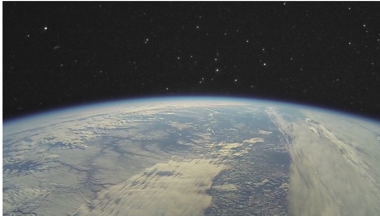
Figure 27: Horizon in the FOV is a problem for the star tracker. The picture is a composition of an image of earth taken from MUSCAT Experiment [15] and a star picture taken with the actual image sensor for the star tracker.
