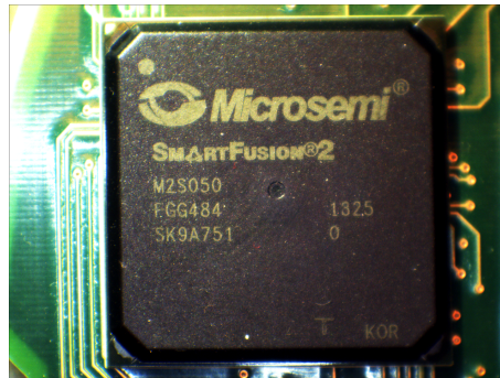
Figure 8: M2S050 Smartfusion2 SOC used for LISA and tracking.
