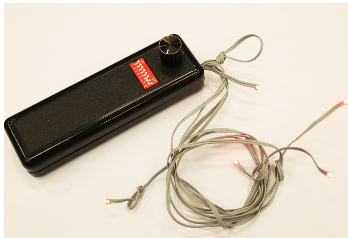
Figure 19: Rechargeable light source with adjustable intensity to simulate stars.
