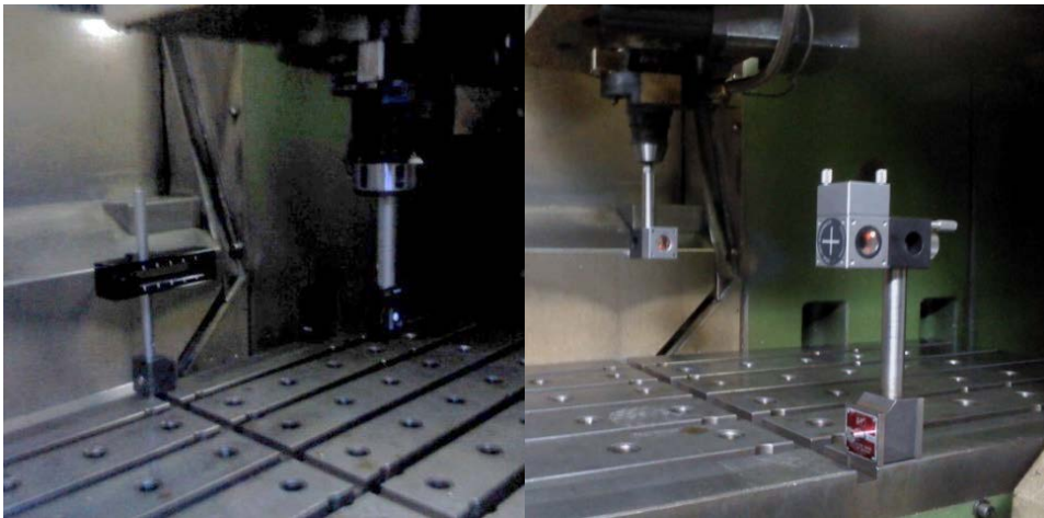
Figure 17. Measurement of the horizontal straightness of the Y axis (left). Straightness reflector was located on the middle line of the machine table and the position was roughly recorded. On the right, the linear positioning measurement of the Y axis can be seen.
