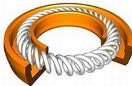
Figure 2.3.2 Garter spring seal
