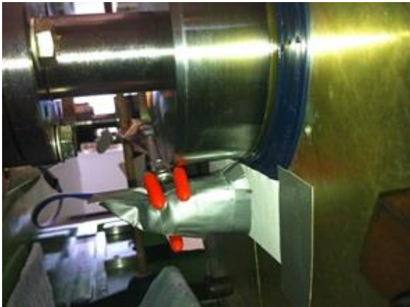
Figure 3.1.19 Photoreflexor attached to the test rig
