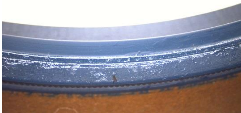
Figure 4.3.1 Enlarged view of leaked seal lip
