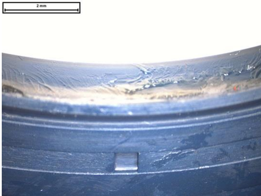
Figure 4.3.2 Enlarged view of un-leaked seal lip
