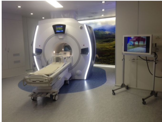
Figure 3: 3T MRI system, GE Healthcare Discovery MR750W, USÖ. Photography by Adam Trowald.
