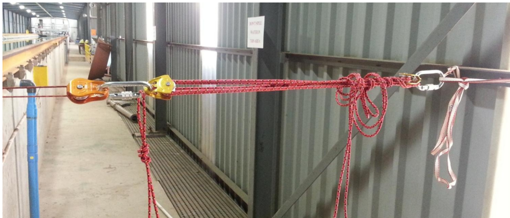
Figure 3.5 – The pulley system attached to the wall.
