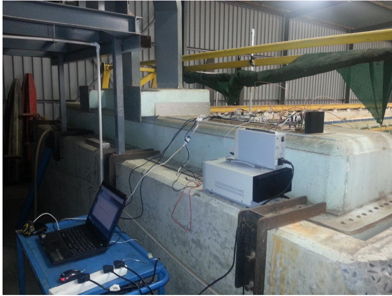
Figure A.1 – The laptop, power supplies and SONAR equipment set up at the towing tank.
