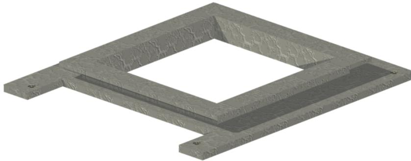
Figure 4.8: Air coil magnetorquer structure prototype
