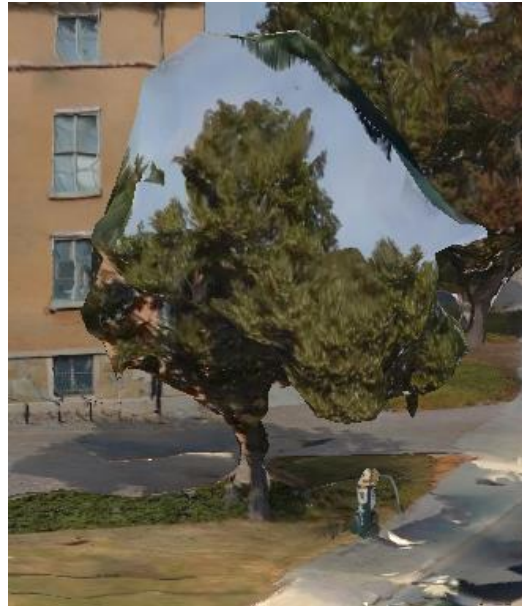
Figure 34 Screenshot in Smart3DCapture, tree reconstructed from street view and aerial images
