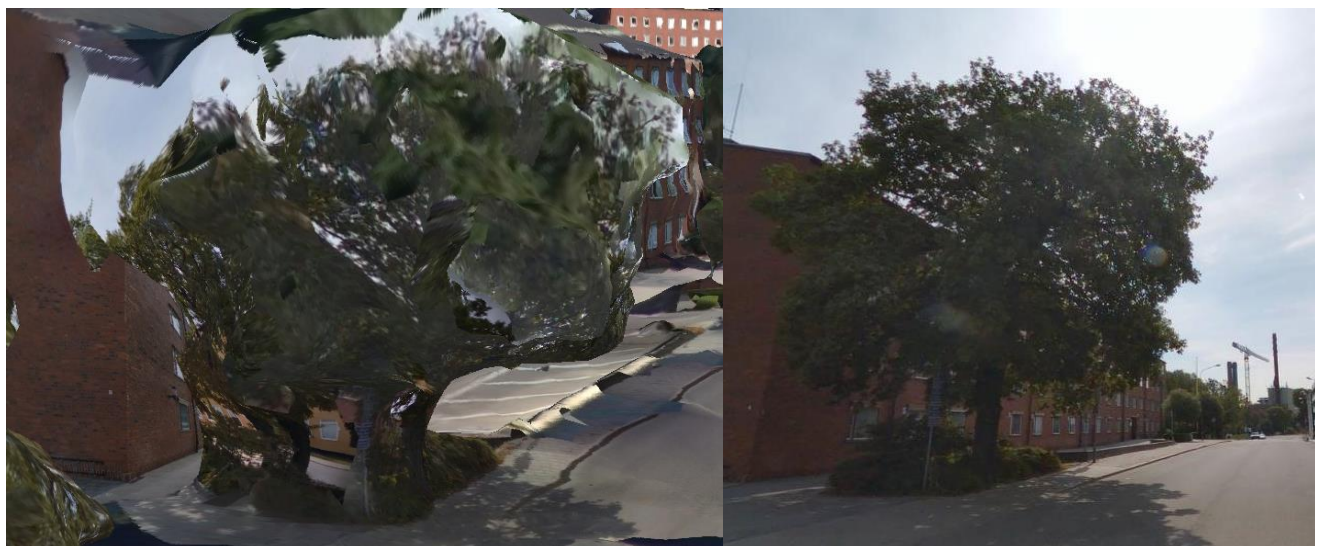
Figure 35 Faulty tree based on street view images (left), screenshot Smart3DCapture and original image of the tree (right), Cyclomedia
