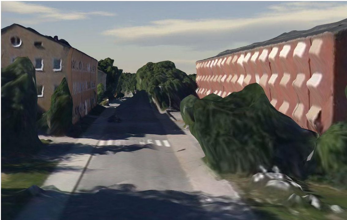
Figure 20 Screenshot in Smart3DCapture, street view of the model reconstructed from aerial images
