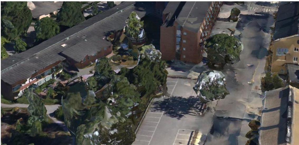
Figure 41 Screenshot in Smart3DCapture of model reconstructed from aerial and street view images
