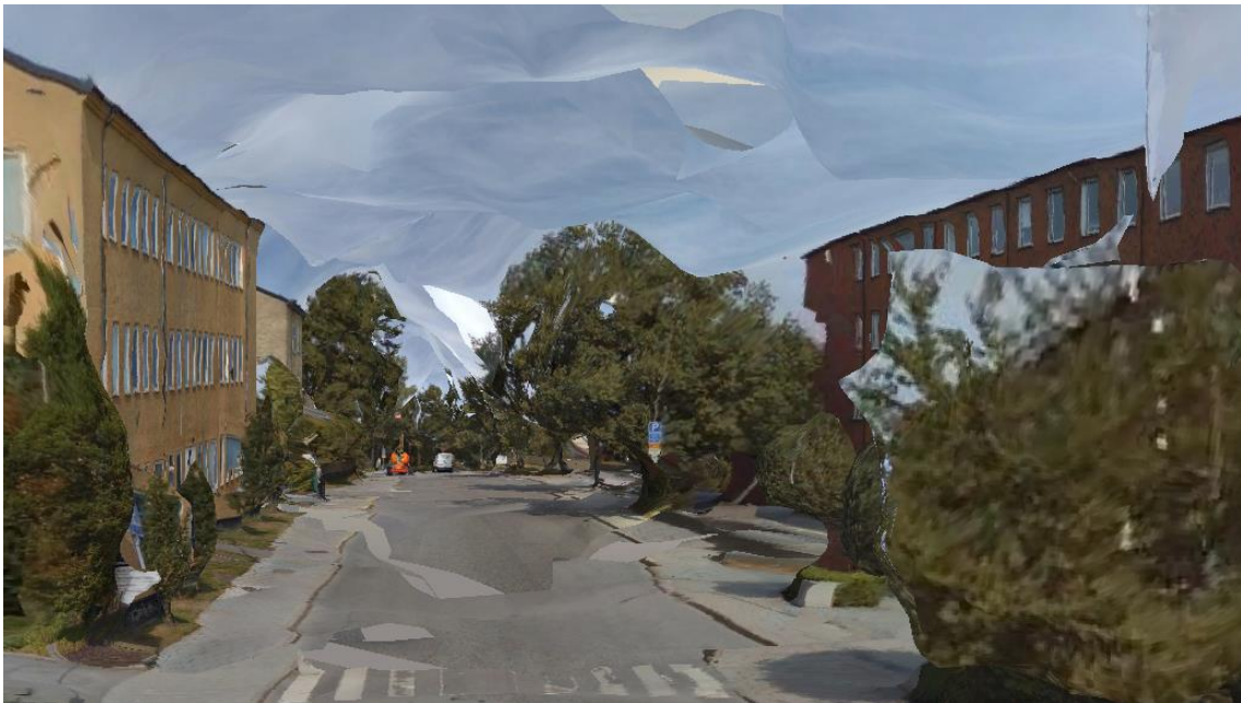
Figure 24 Screenshot in Smart3DCapture, model reconstructed from street view images
