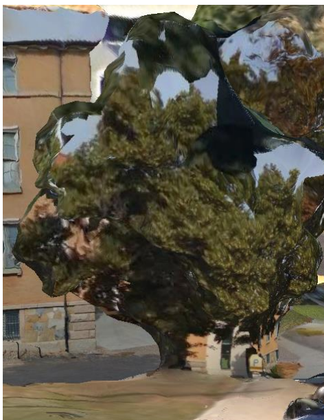
Figure 36 Screenshot in Smart3DCapture, tree reconstructed when importing aerial images first
