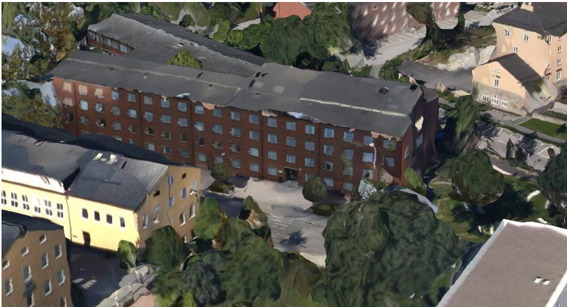
Figure 31 Screenshot in Smart3DCapture, model reconstructed from aerial and street view images
