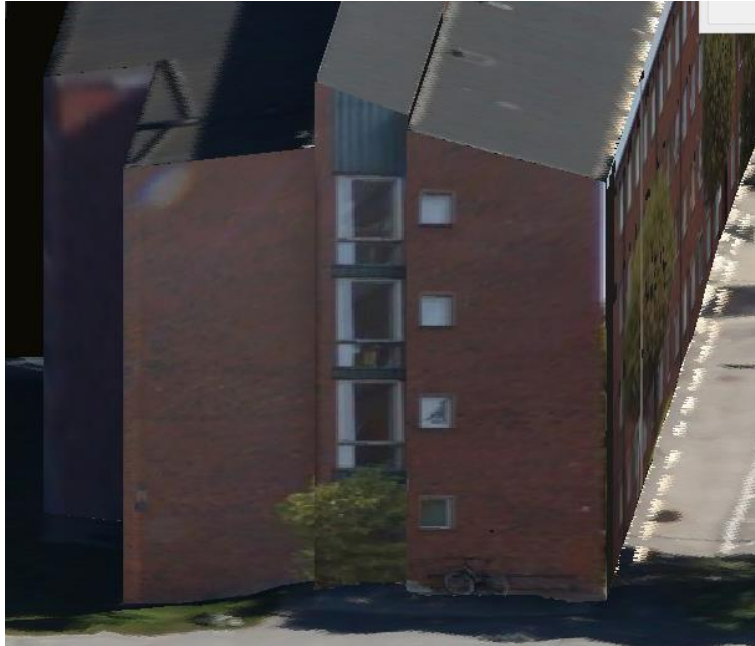
Figure 15 Screenshot in TerraPhoto, automatically chosen texture for the building façade
