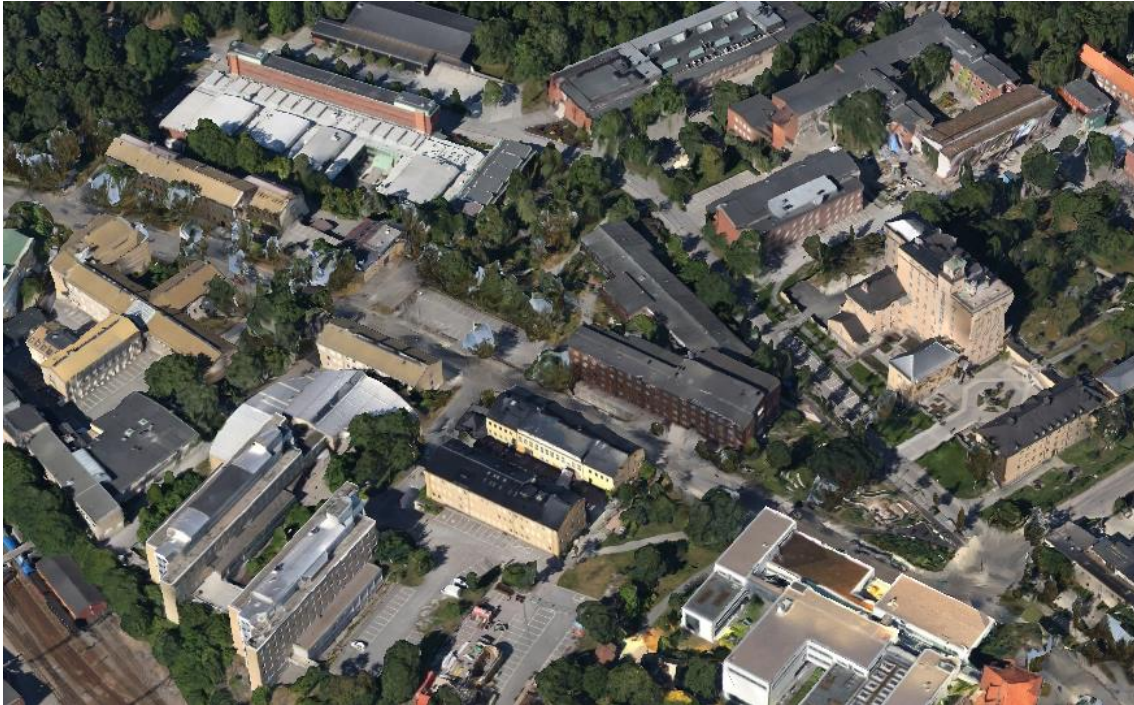
Figure 30 Screenshot in Smart3DCapture, reconstructed model with both aerial and street view images seen from above
