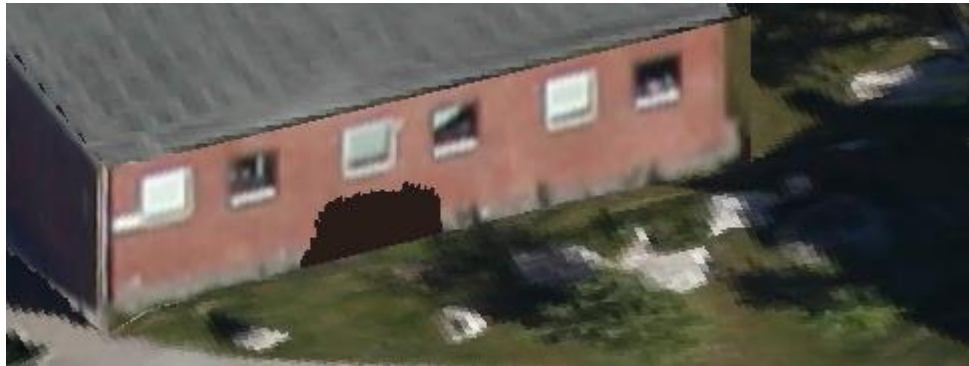
Figure 5 Screenshot in TerraPhoto, hole in the façade due to the use of depth maps
