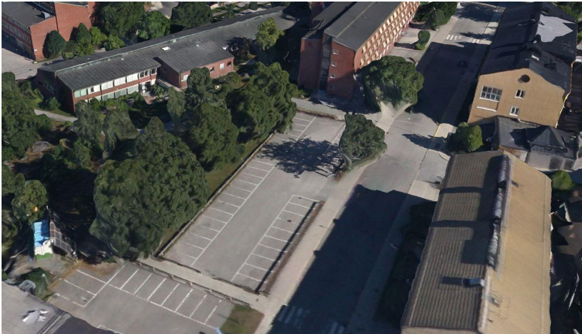
Figure 40 Screenshot in Smart3DCapture of model reconstructed from aerial images
