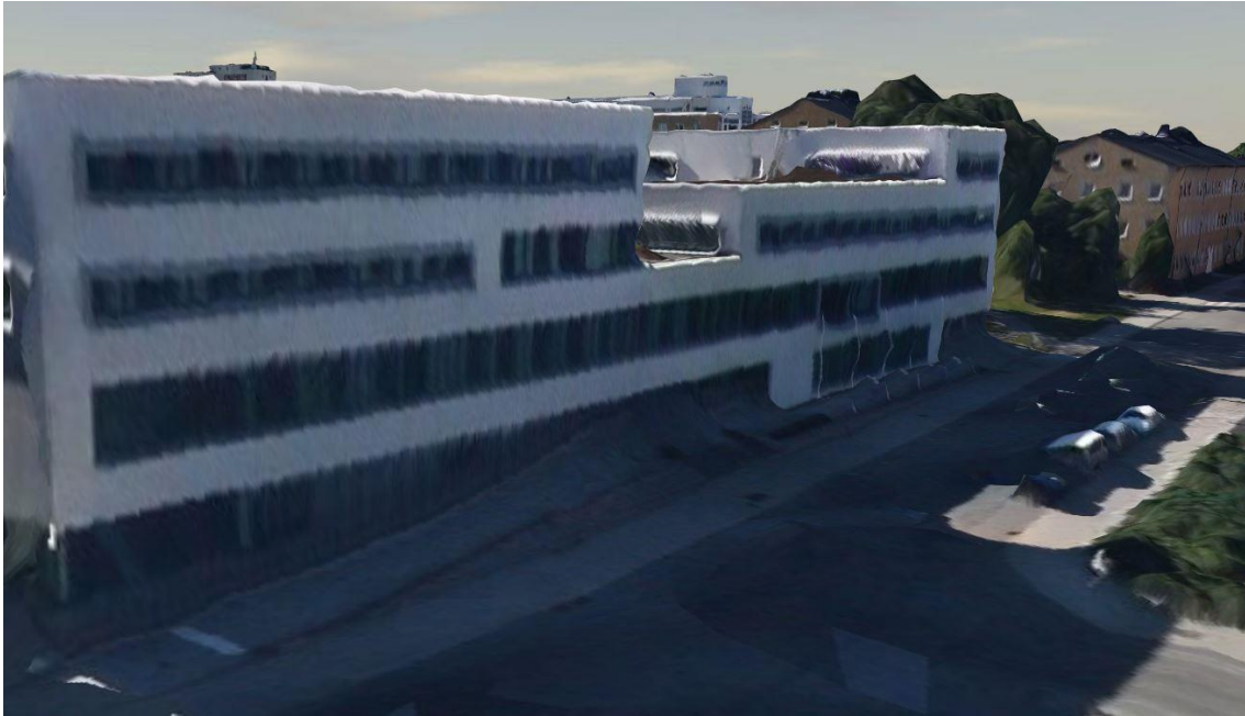
Figure 22 Screenshot in Smart3DCapture, blurry façade in model reconstructed from aerial images
