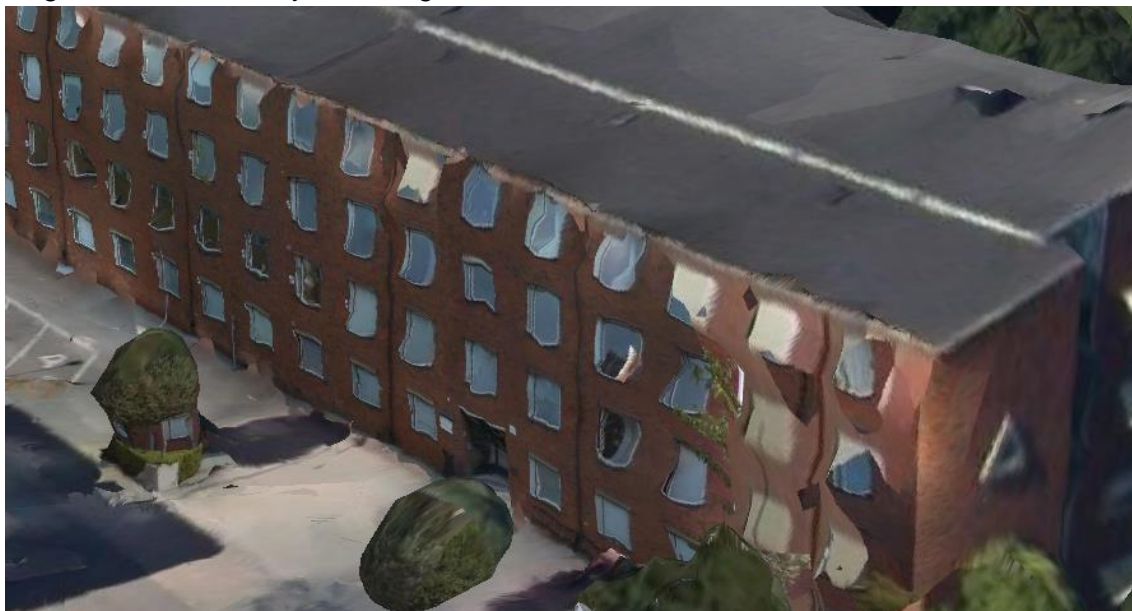
Figure 37 Screenshot in Smart3DCapture, model reconstructed with images imported in reversed order
