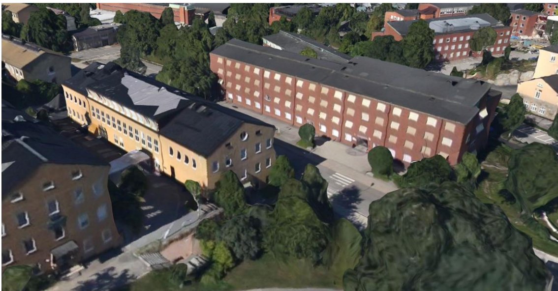
Figure 19 Screenshot in Smart3DCapture, overview of model reconstructed from aerial images
