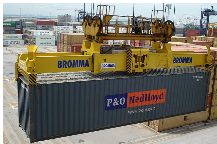
Figure 2.1. Example of a Bromma spreader lifting a container (Credit1Coach, 2012)
