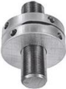
Figure 2.24. A typical spiral washer for a laboratory fatigue testing machines
