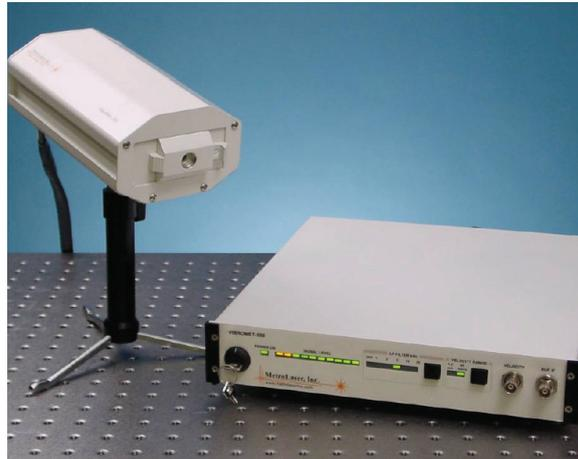
Figure 3.3: The MetroLaser Inc. Laser Doppler Vibrometer 500V used in the study. By directing the laser beam at the participant's chest wall, a velocity profile related to the underlying mechanics of the heart can be detected (MetroLaser Inc., 2010).
