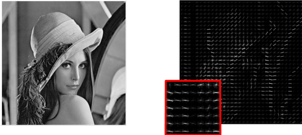
Figure 2.3: The image to the right shows the corresponding gradients of the cells. Each cells histogram, that is the different intensity gradient bins, are represented as lines where one line correspond to one angular bin and the length of the line correspond to the size of that bin. The image to the right also shows a square that have been enlarged which shows part of the HOG grid containing 7 by 7 cells.
