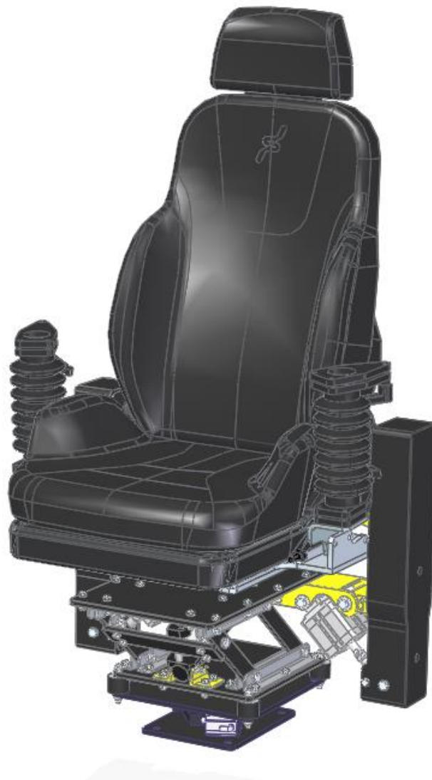
Figure 51: CAD-model of an operator seat mounted on the final undercarriage design.
