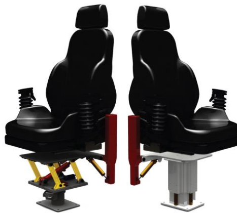
Figure 2: Operator seat design concepts (Doroftei & Osario, 2013).
