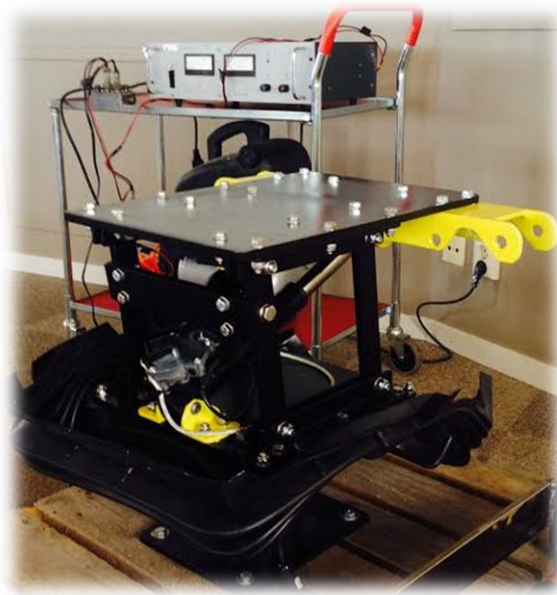
Figure 61: Half-assembled prototype connected to a 24VDC electric box for demonstration.
