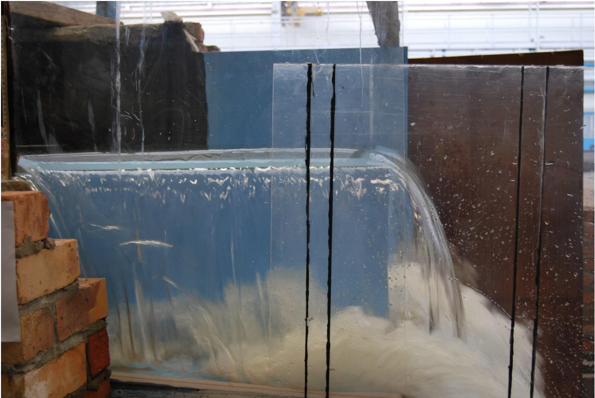
Figure C.7 Labyrinth weir side view under low flow conditions, showing aeration conditions, surcharge level and flow patterns
