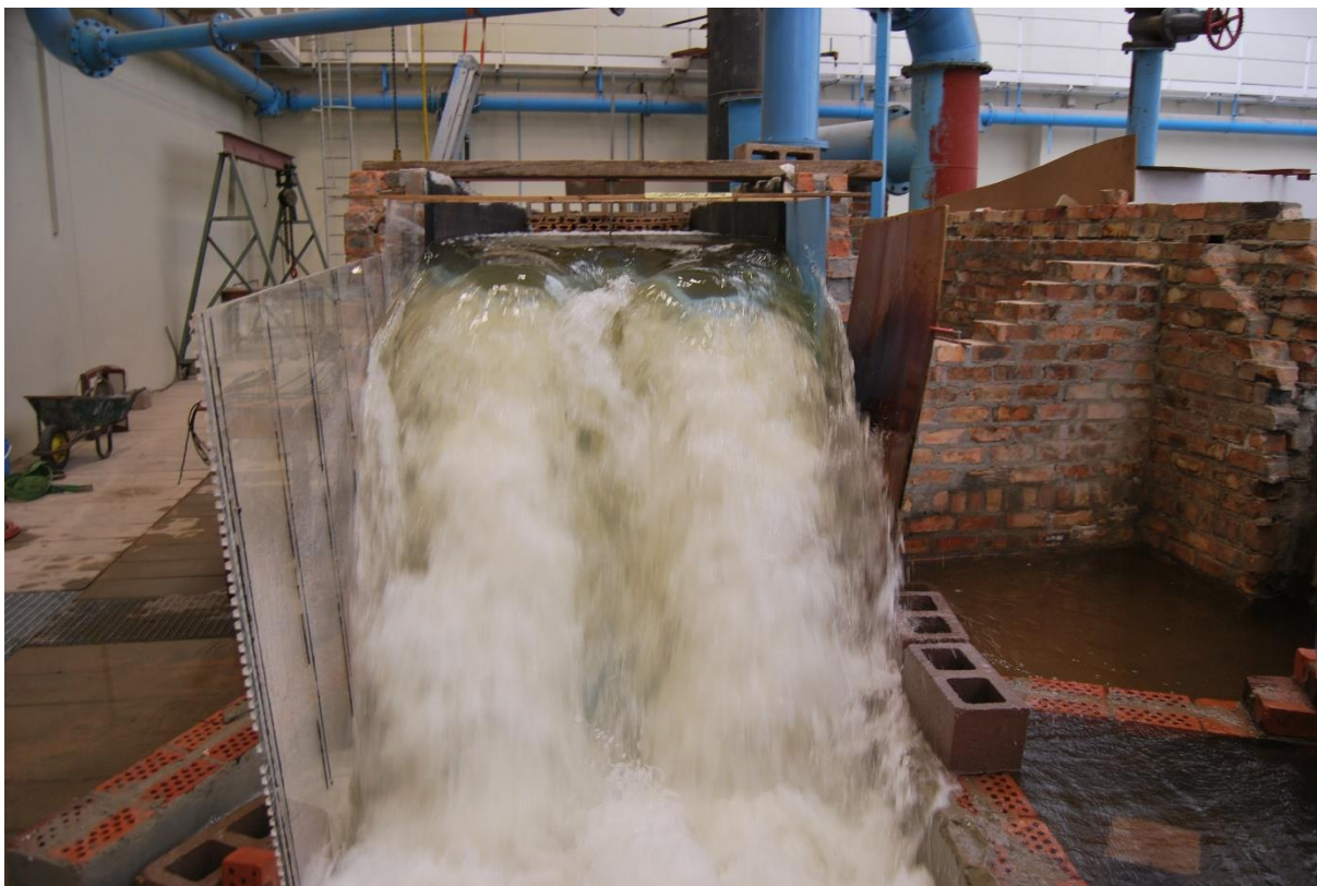
Figure C.14 Labyrinth weir viewed from downstream under high flow conditions, showing aeration conditions, turbulence and flow patterns
