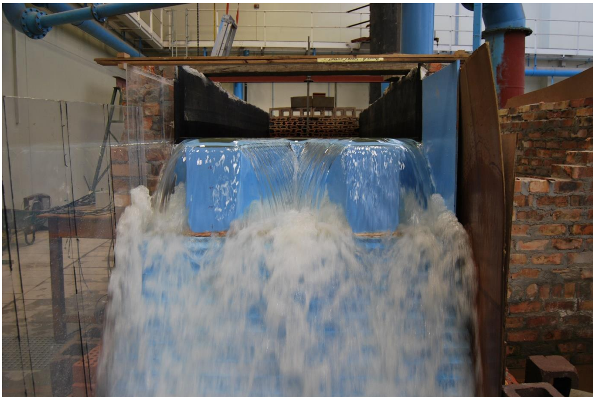
Figure 4.15 Physical model of labyrinth weir with a discharge of 60 l/s at a scale of 1:20, viewed from downstream (215 m 3 /s discharge at the prototype scale, at a unit discharge of 3.6 m 3 /s-m)
