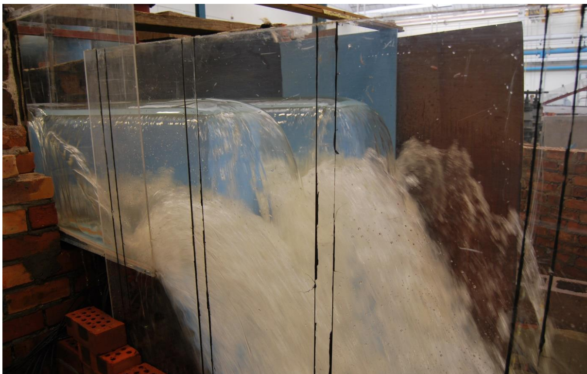
Figure 5.18 Physical model aeration and flow behaviour under low discharge conditions of 544 \text{ m}^3/\text{s} ( 153 \text{ l/s} at a scale of 1:20)
