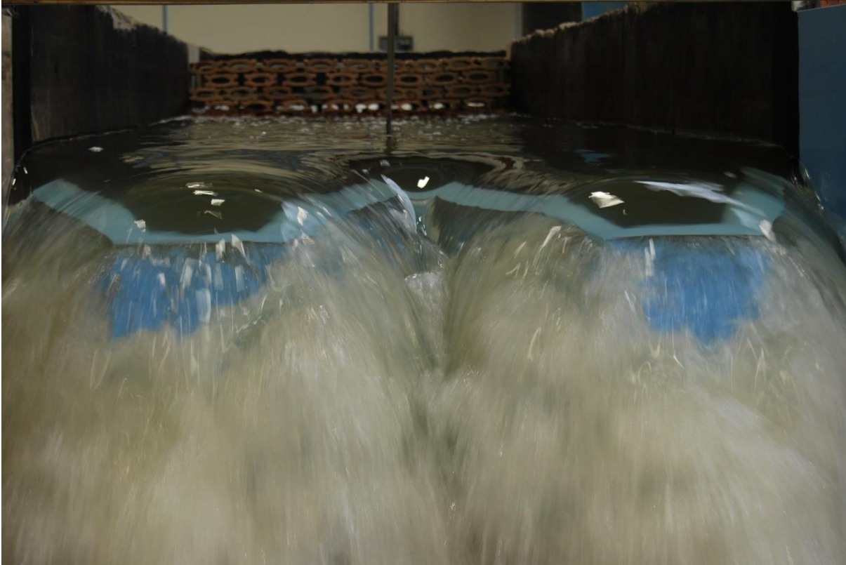
Figure 4.17 Physical model of labyrinth weir with a discharge of 297 l/s at a scale of 1:20, viewed from downstream (1 063 m 3 /s discharge at the prototype scale, at a unit discharge of 17.7 m 3 /s·m)
