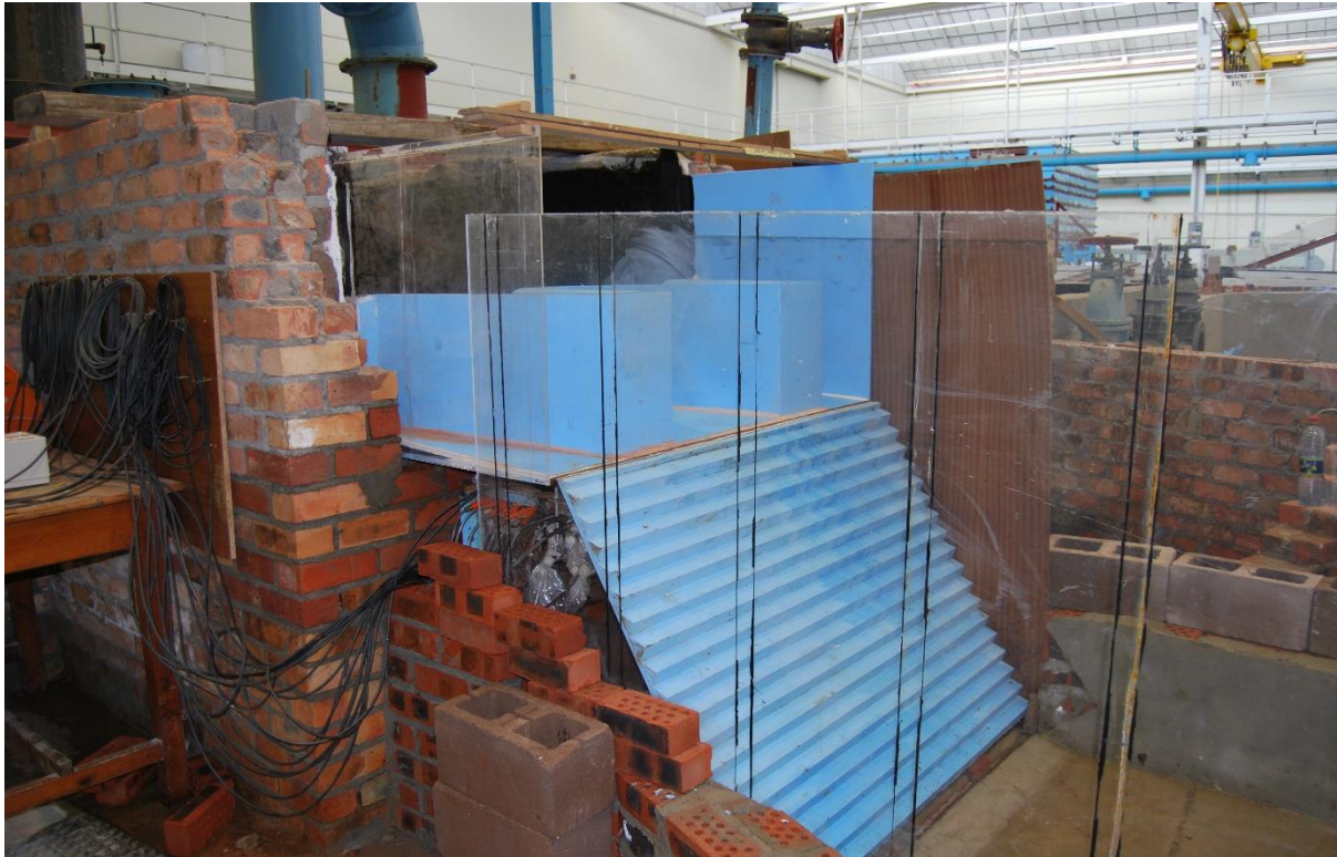
Figure C.1 Physical model viewed from downstream showing Perspex side walls and pressure sensor cables coming out from underneath the model
