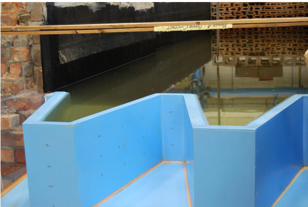
Figure C.4 Labyrinth weir crest viewed from downstream, showing water in the flume at the crest level and pressure sensor positions on the downstream crest face
