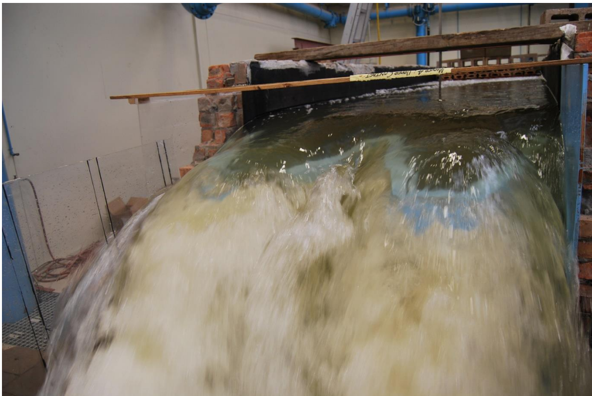
Figure 4.19 Physical model of labyrinth weir with a discharge of 597 l/s at a scale of 1:20, viewed from downstream (2 136 m 3 /s discharge at the prototype scale, at a unit discharge of 35.6 m 3 /s-m)
