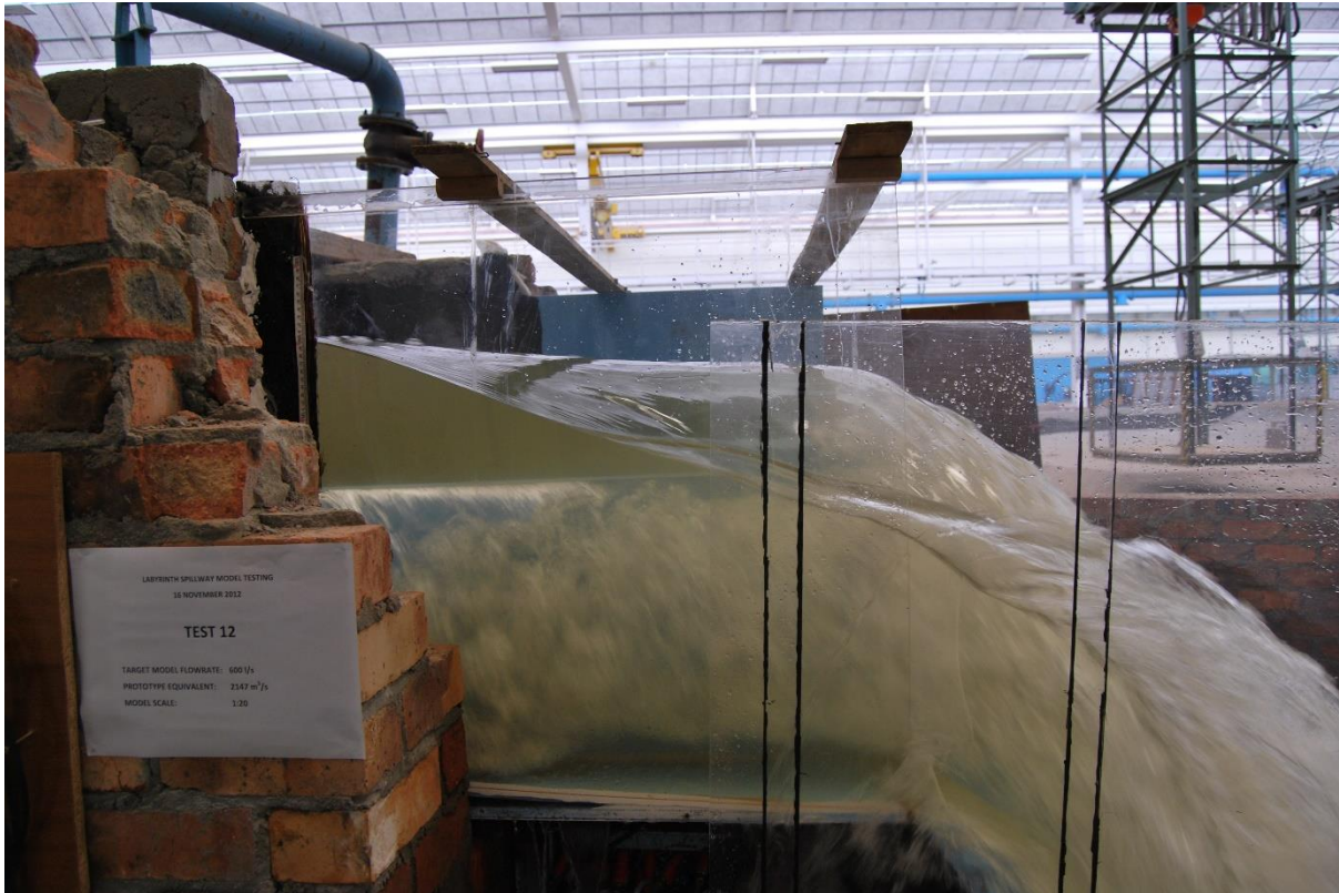
Figure C.13 Labyrinth weir viewed from the side under high flow conditions, showing surcharge and aeration conditions
