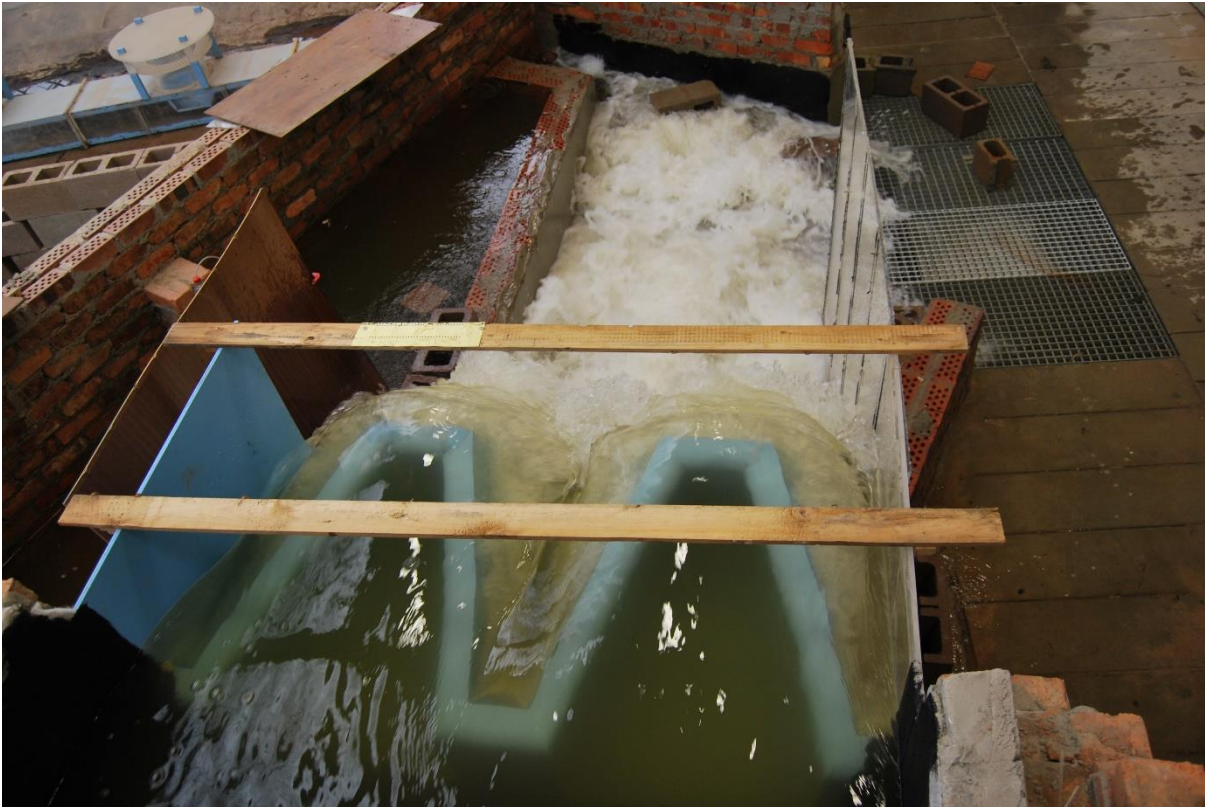
Figure 4.18 Physical model of labyrinth weir with a discharge of 597 l/s at a scale of 1:20, viewed from above (2 136 m 3 /s discharge at the prototype scale, at a unit discharge of 35.6 m 3 /s-m)
