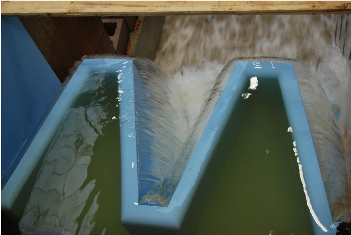
Figure 4.14 Physical model of labyrinth weir with a discharge of 60 l/s at a scale of 1:20, viewed from above (215 m 3 /s discharge at the prototype scale, at a unit discharge of 3.6 m 3 /s-m)
