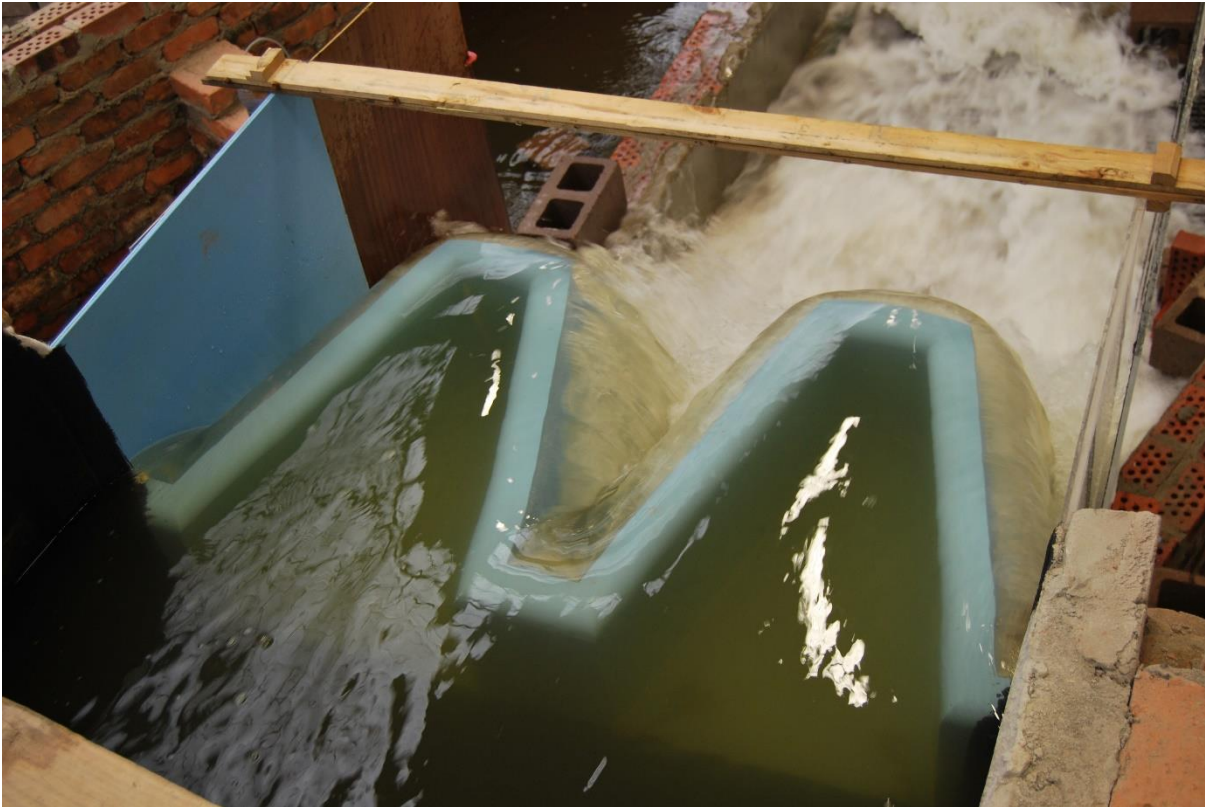
Figure C.9 Labyrinth weir model viewed from above under medium flow conditions, showing flow patterns and aeration conditions
