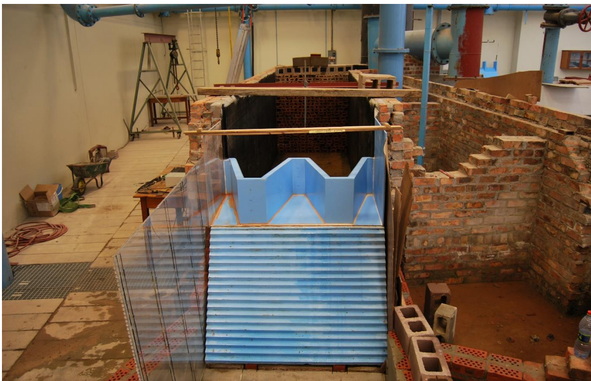
Figure C.2 Labyrinth weir model viewed from downstream showing weir crest, flume and baffle wall at upstream section of flume
