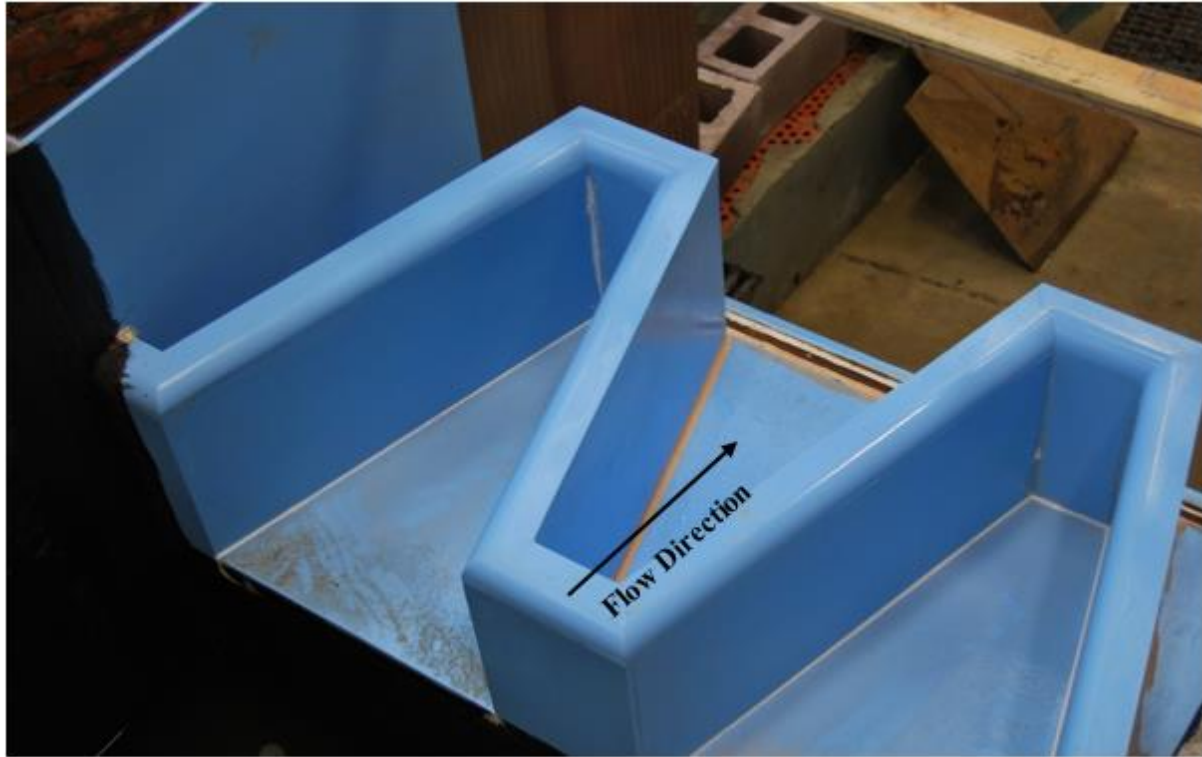
Figure 4.2 View of model constructed, from above and upstream of the crest
