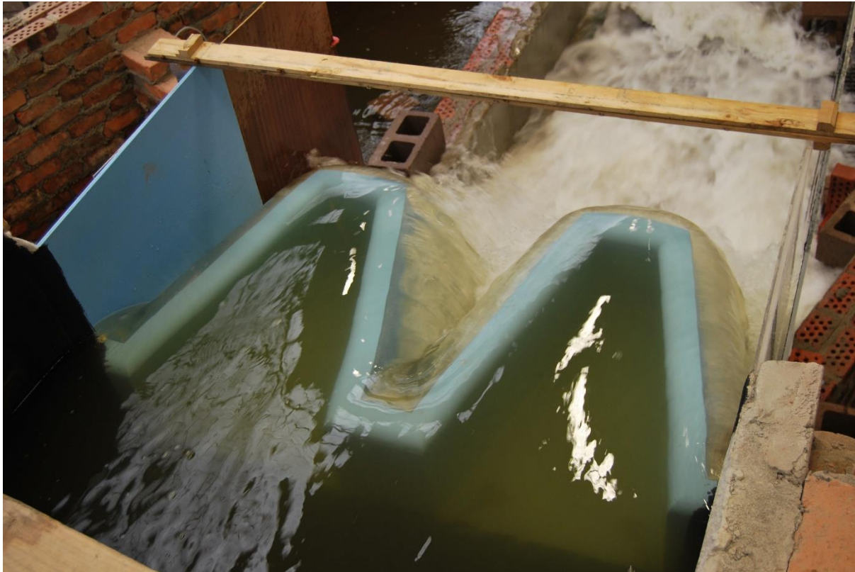
Figure 5.20 Physical model aeration and flow behaviour under medium discharge conditions of 1\ 063\ \text{m}^3/\text{s} (297 l/s at a scale of 1:20)
