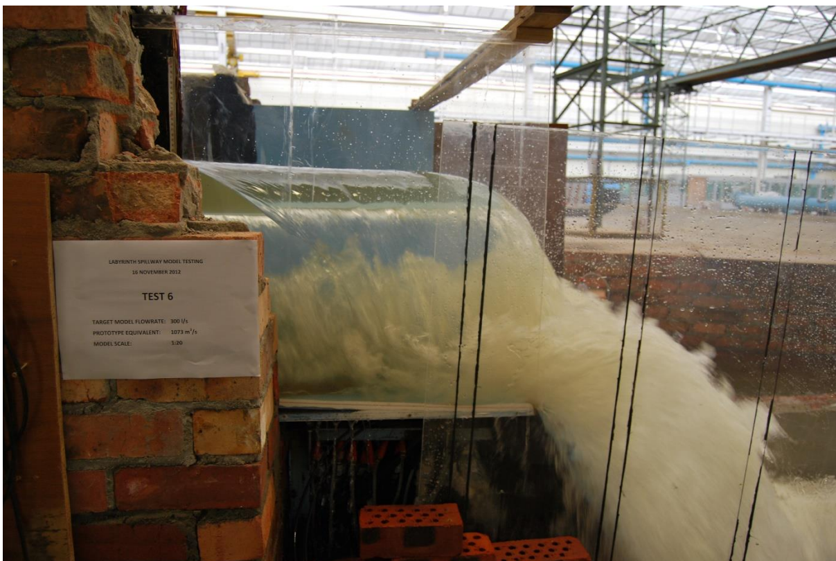
Figure C.10 Labyrinth weir viewed from the side under medium flow conditions, showing surcharge and aeration
