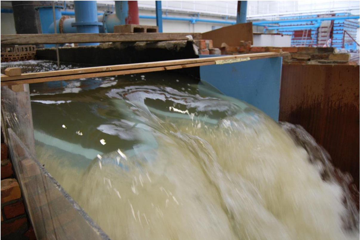
Figure C.11 Labyrinth weir viewed from downstream under high flow conditions, showing flow patterns and aeration conditions
