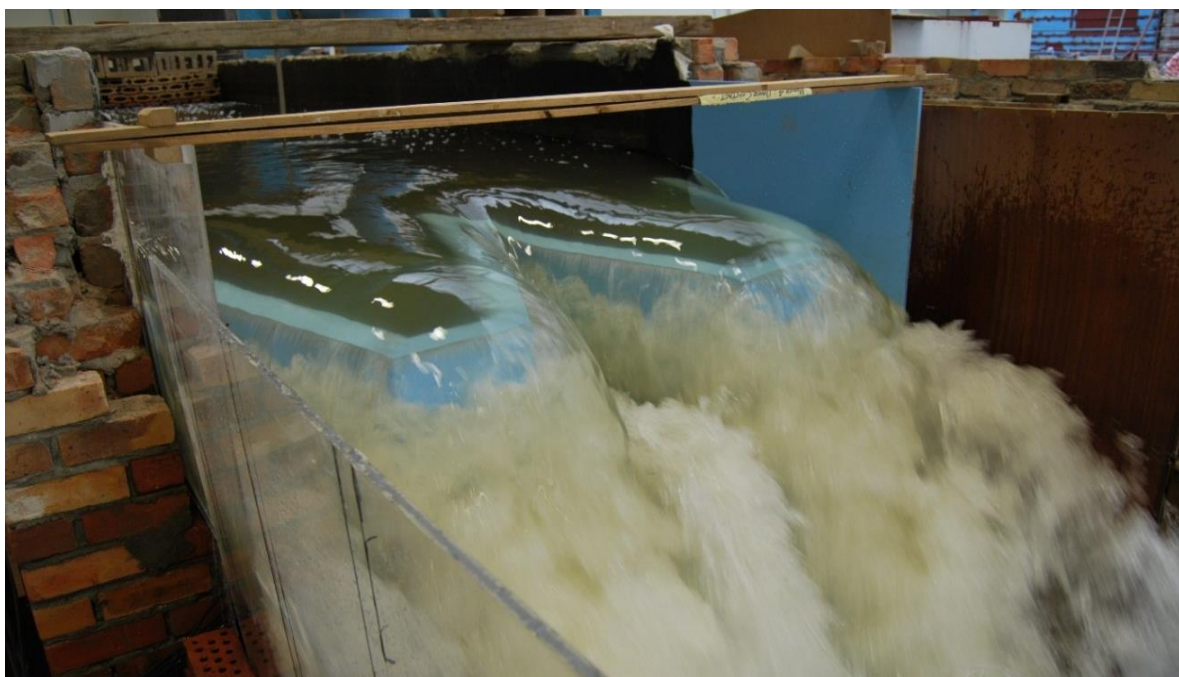
Figure 5.16 Physical model aeration and flow behaviour under high discharge conditions 1 606 m 3 /s (450 l/s at a scale of 1:20)
