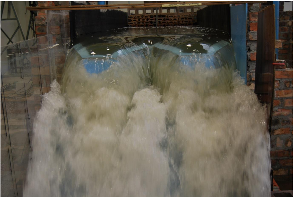
Figure C.8 Labyrinth weir viewed from downstream under medium flow conditions, showing turbulence, aeration and flow patterns
