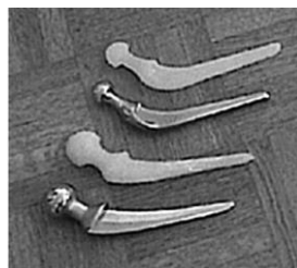
FIG. 9: Metal orthopaedic implants (hip arthroplasty) and corresponding wax replica [Adapted from Kolind et al.2004].
