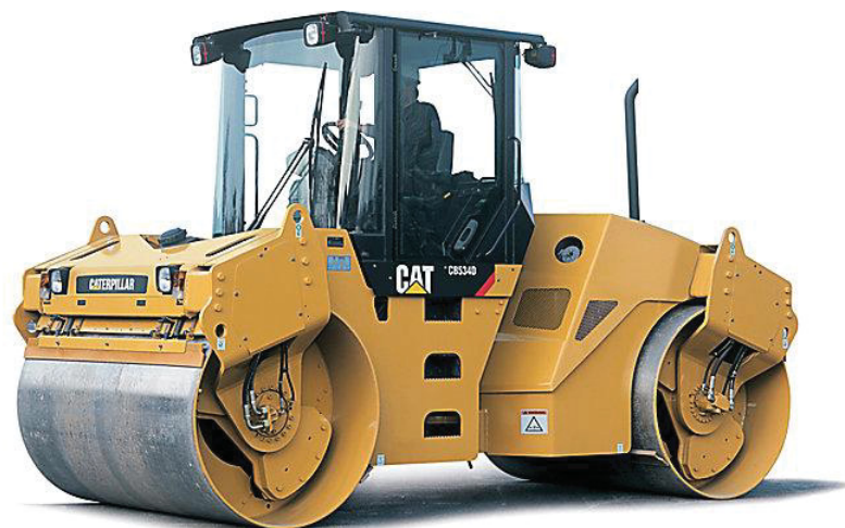
Figur 4.3 picture of Cat tandem roller. The lower scraper can be seen on both wheels.(12)
