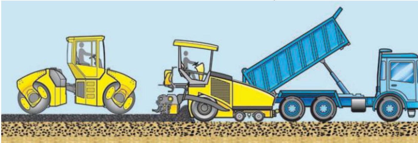
Figure 2.2 (3) Picture of the compaction can look like. To the left we have an roller which could be an tandem roller. Next in the middle we have the finisher who is laying out the asphalt and make some compaction. Last we have a truck that unloads an steady stream of material into the finisher.
