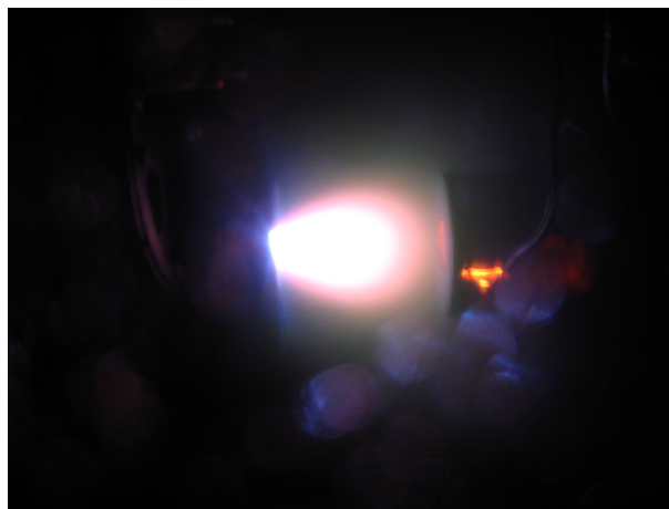
Figure 4.5: Laser ablated plasma plume from a stoichiometric YBCO target in a 0.08mbar oxygen ambient environment.
