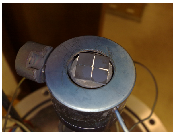
Figure 4.6: Photo of the custom built substrate heater [29], with four samples mounted with conductive silver paint. The temperature probe enters through the heat shield (bottom middle).
