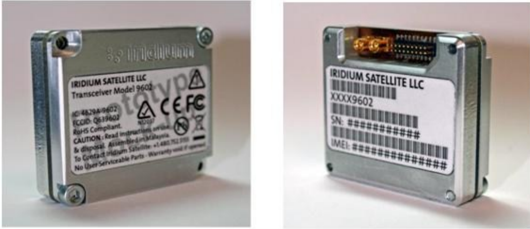
FIGURE D.1: 9602 Iridium modem.
