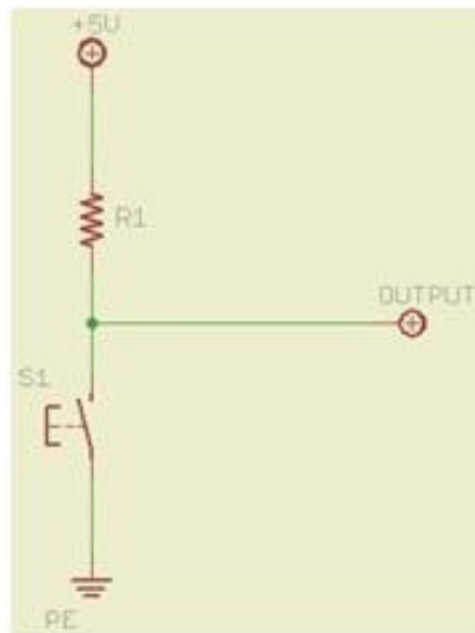
FIGURE 3.15: Pull up resistor configuration.
