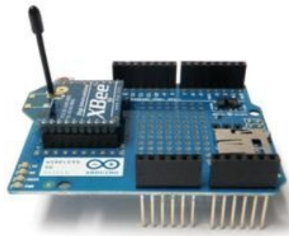
FIGURE 4.2: Microcontroller transceiver interface.
