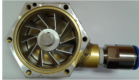
Figure 3.18: CNC milled rotor fitted inside the turbine casing
