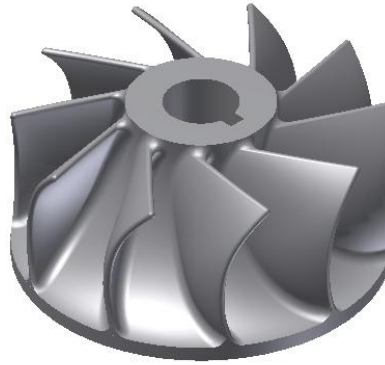
Figure 3.13: Rotor CAD model (Autodesk Inventor Professional 2011)
