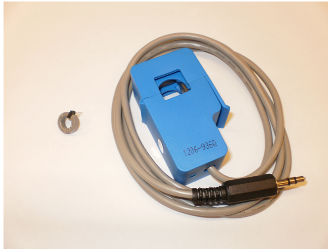
Figure 28. The Hall sensor is the smaller one on the left and the current transformer with the clamp is on the right.
