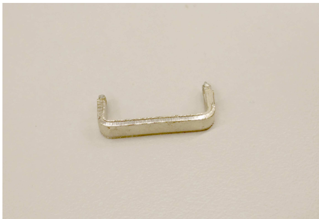
Figure 2. A piece of metal used as a shunt resistor in a cheap commercial energy meter.
