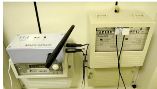
Figure 15. The mains sensor of the UBI-AMI version 1. Below the sensor box is the optical pulse input.
