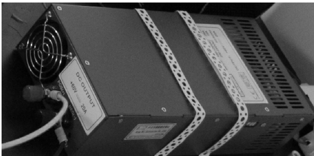
Figure 37: The rectifier used in the prototype system
