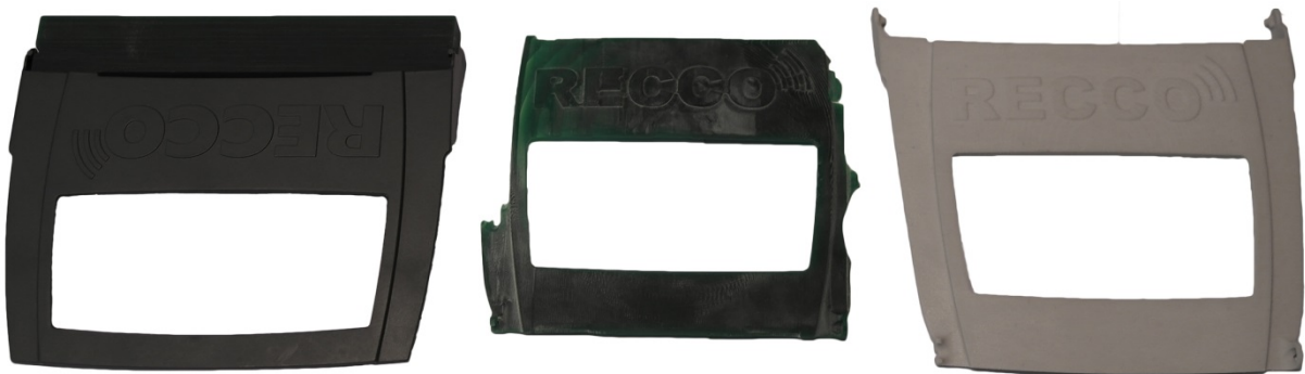
Figure 4. Different kind of both successful and not so successful prototypes of the antenna.
