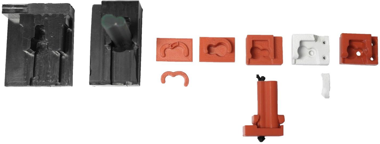
Figure 7. The snap fit antenna's snap fits development from left to right.
