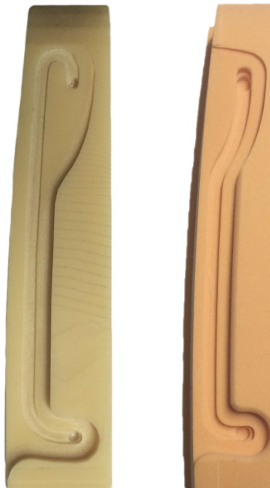
Figure 23. Two different prototypes of the sliding mechanism, the left one is the initial design and the right one the improved.
