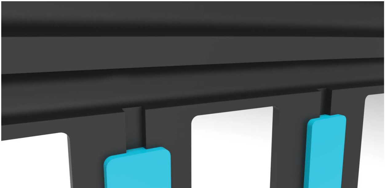
Figure 25. The ventilation canals between the blue directors and the inner sweep canal.
