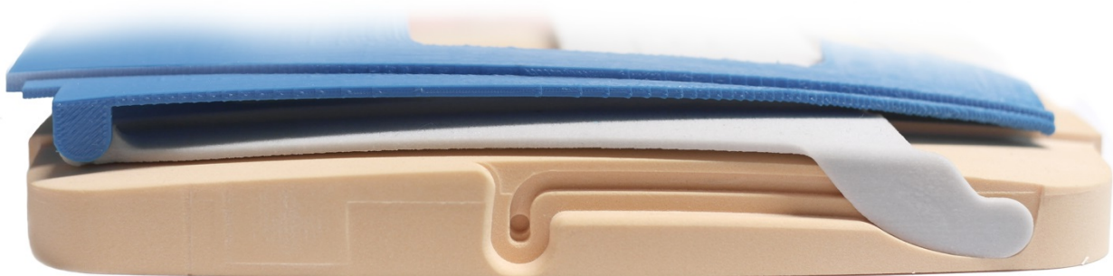
Figure 2. The sliding concept folded in profile; the orange on the bottom is the detector then comes the off-white first antenna part and then the blue outer antenna part.
