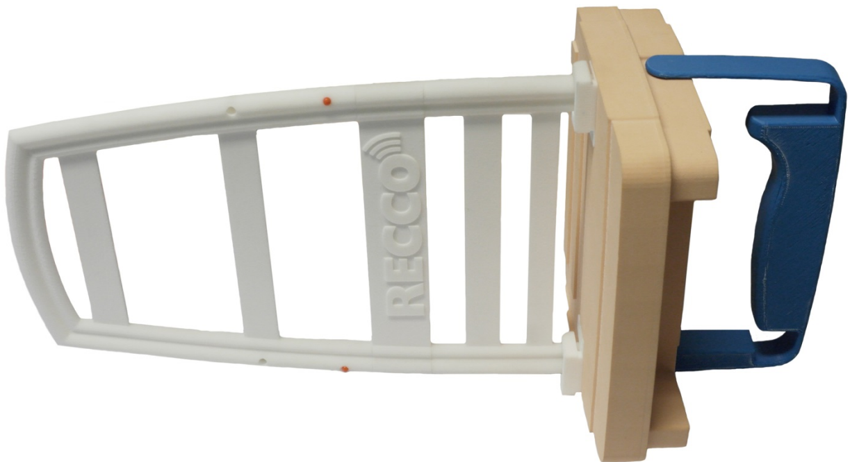
Figure 40. The final prototype of the antenna in extended position.
