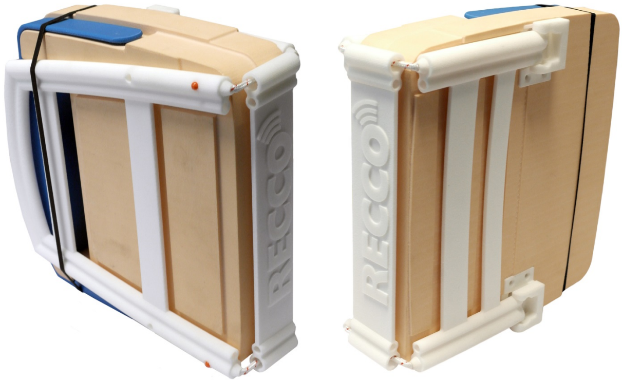
Figure 41. The prototype of the antenna in folded position.
