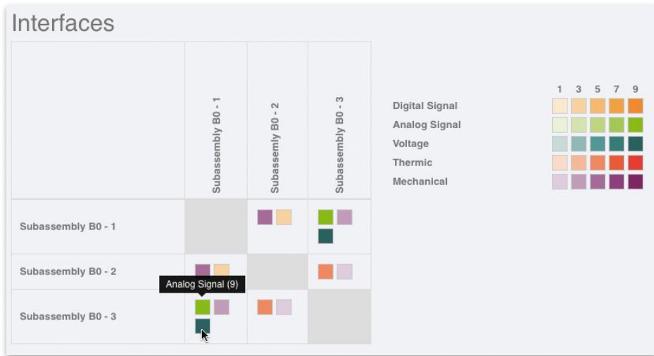
Figure 62. Interfaces represented with color-coded boxes in a dependency matrix.
