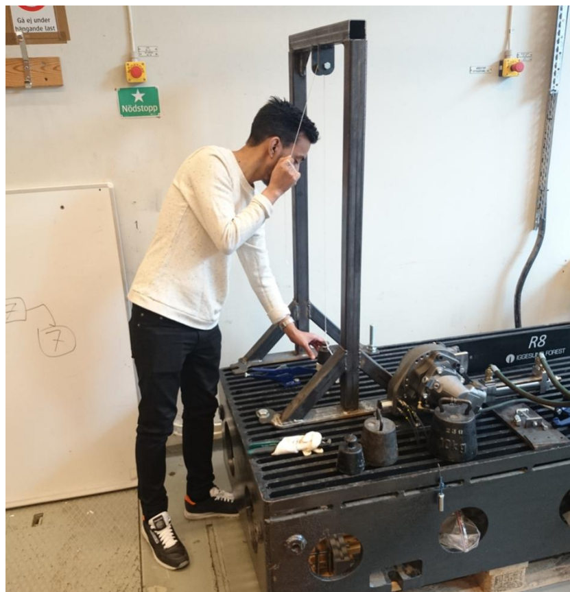
Figure 24. Drop test construction.
