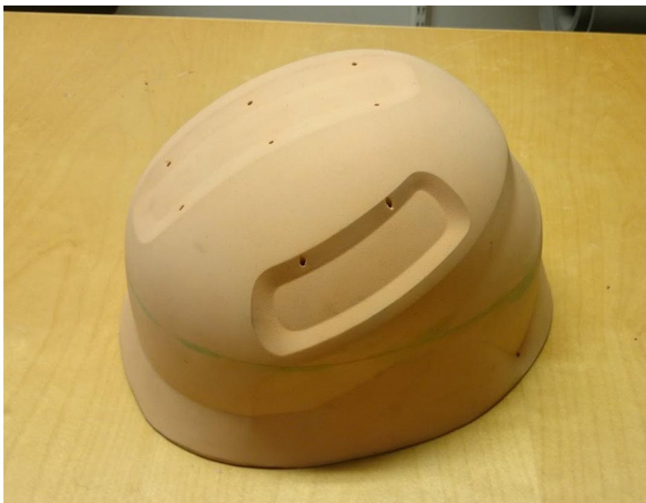
Figure 67. Mould used for vacuum forming the outer shell.
