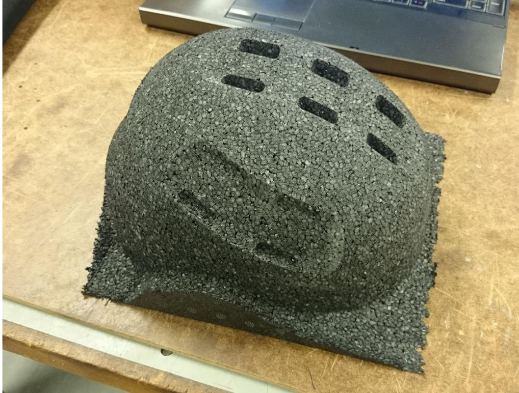
Figure 70. Milled outer surface of inner liner.
