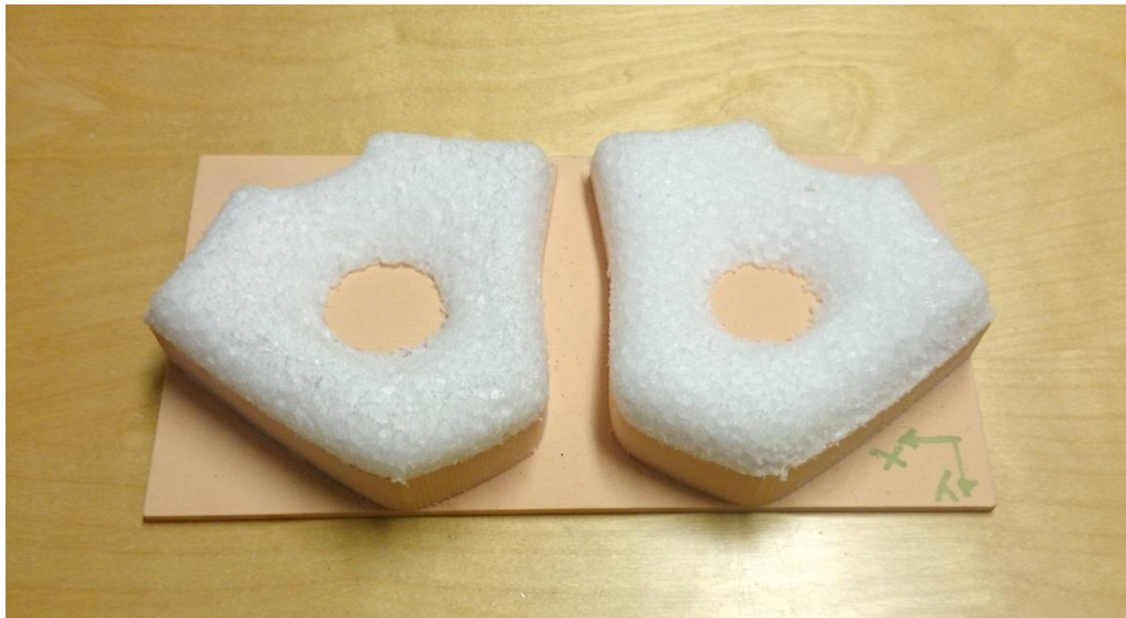
Figure 73. EPP liners for ear cover, with CNC fixture.
