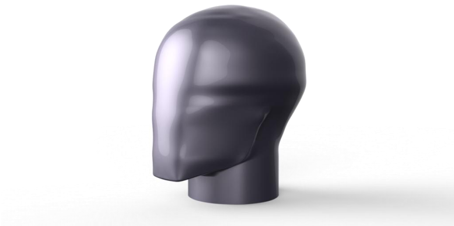
Figure 34. CAD model of EN960:1995 head form, size J.
