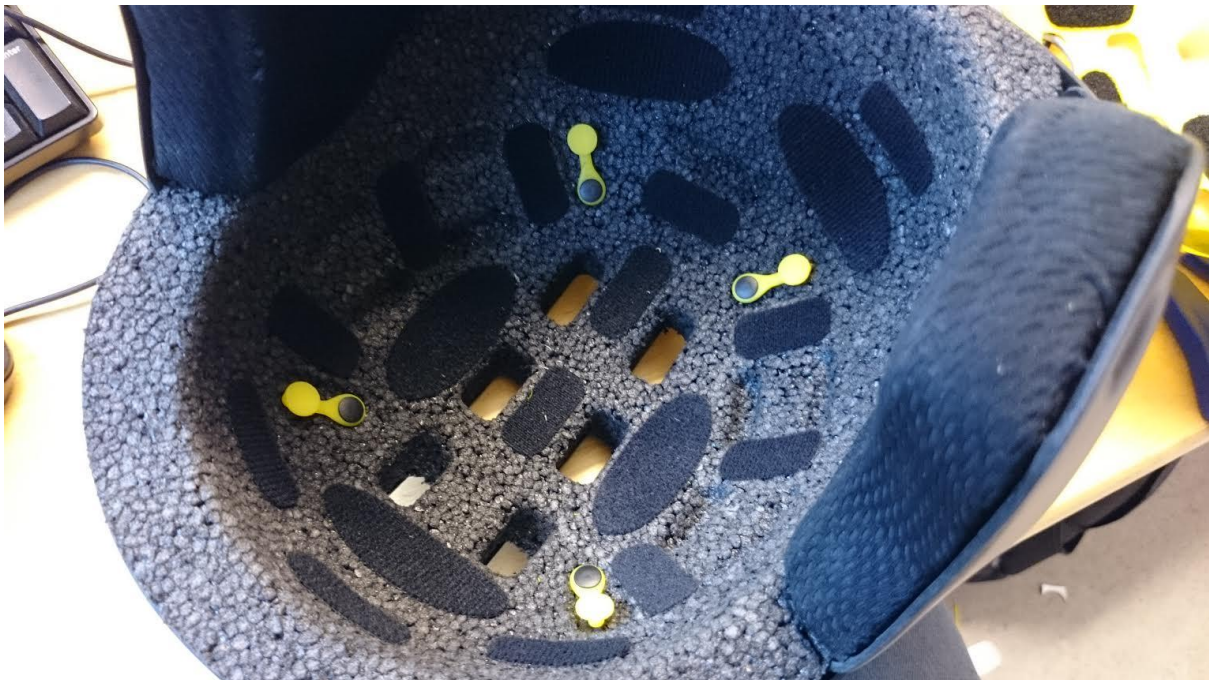
Figure 77. Liner inside with MIPS low friction pads.
