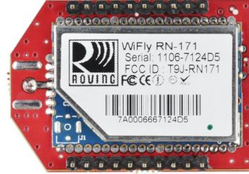
(b) The WiFi module from Roving Networks the breakout board used.
