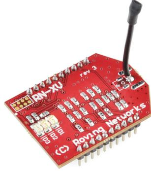
(a) The breakout board from Sparkfun with a wire antenna.
