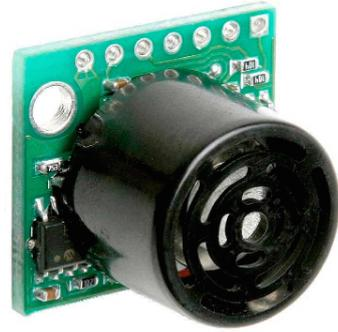
(b) The ultrasonic sensor used, LV-EZ3 from Maxbotix.<sup>1</sup>
