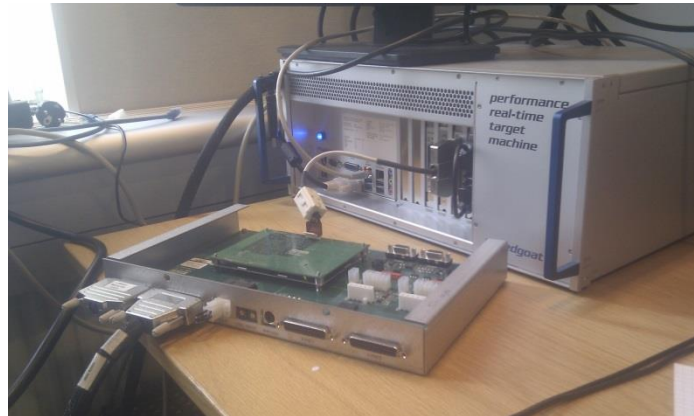
Figure 4: CMOT3 unit, here connected to a Speedgoat real-time computer with an SPI cable. The UNIX computer, which handles commands and other related tasks, is not in the picture.
