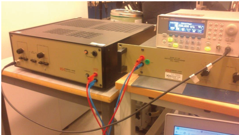
Fig 5.5. Amplifier, Matching Transformer and Signal Generator.
