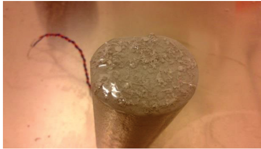
Figure 5.4. Introduction of Unmixed Granulate defect.
