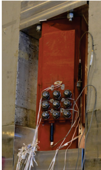
Figure 8.1 – Apparatus of the Finger Connection Compression test
