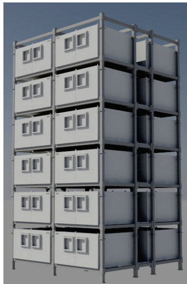
Figure 1.1: 3D modules sited on the steel framed structure
