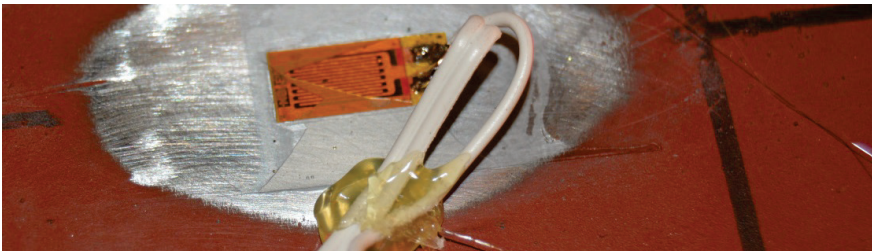
Figure H.3: Strain Gauge installed in Finger Plate
