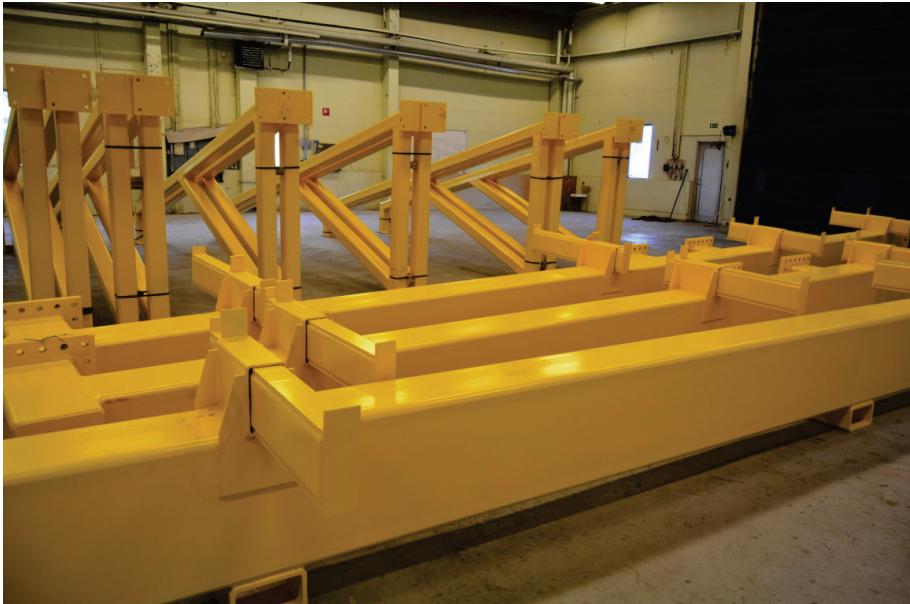
Figure F.4: Full scale test – installation of the Lifting system
