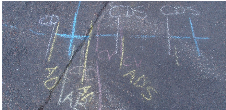
Figure 30 An example of the marks painted on the ground to show where the experienced gaps are and a-pillars are situated.
