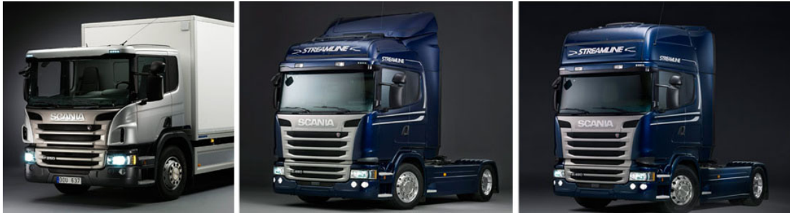
Figure 10 Scania P-, G- and R-series with different height configurations (image courtesy of Scania).
